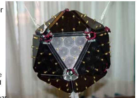
Berkeley Center for New Music and Audio Technology (CNMAT) created a compact loudspeaker array: 10-inch-diameter icosahedron incorporating 120 tweeters.
