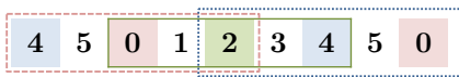
Fig. 6: A 1-dimensional problem space with 6 processors and the cutoff distance b_c = 2 . The red dashed, green solid, and blue dotted frames illustrate the cutoff windows of proc_0 , proc_2 , and proc_4 , respectively.
