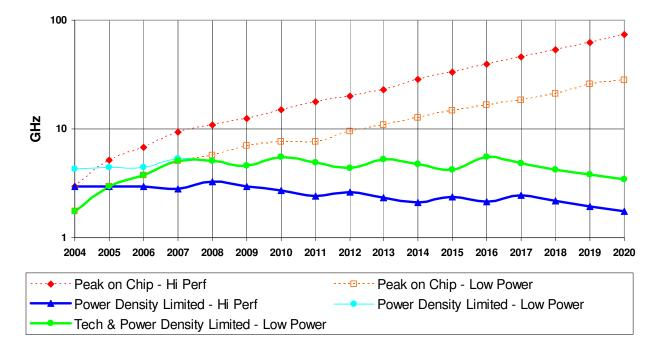
Figure 6.3: Power-constrained clock rate
