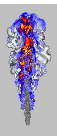
Figure 9: This image shows a developing jet diffusion flame simulation run at NERSC using Berkeley Lab's PeleM code developed as part of the ECP's combustion application project and with adaptive mesh refinement methods and software from the ECP AMReX Co-Design Center. In fluid dynamics problems more broadly, applied math researchers have used optimization, statistical methods and deep learning to aid in parameter estimation and fast surrogates and to derive highly accurate models from data.
