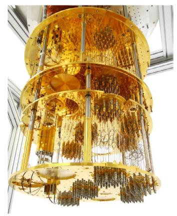
**Figure 22:** Berkeley Lab's Quantum Computing Testbed will include a dilution refrigerator that will house superconducting qubits. Cooling the qubits to a few milliKelvin is required for superconducting to be maintained in the material and to prevent thermal fluctuations from destroying coherence. Photo courtesy of BlueFors Cryogenics.
