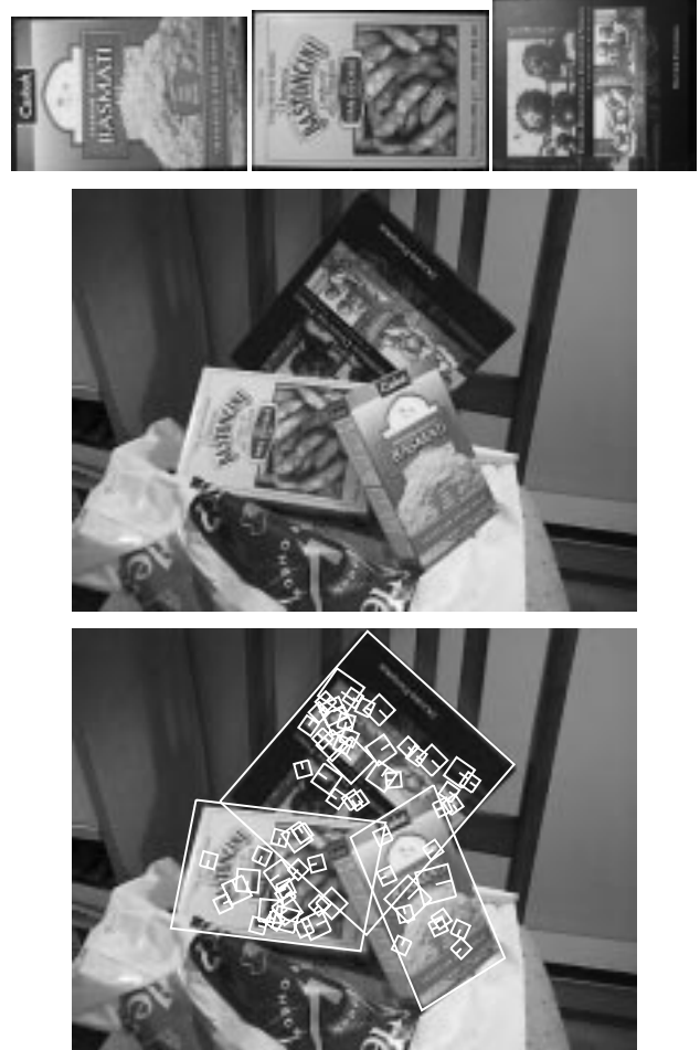
Figure 3: Model images of planar objects are shown in the top row. Recognition results below show model outlines and image keys used for matching.
