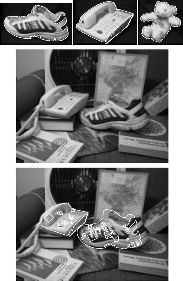
Figure 4: Top row shows model images for 3D objects with outlines found by background segmentation. Bottom image shows recognition results for 3D objects with model outlines and image keys used for matching.
