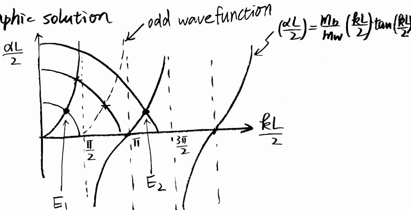
$A_2, B_1$  can be solved by substituting solution  $E_1$  (or  $E_2$ ) in ① (or ②)
