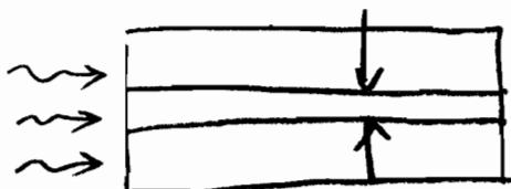
Waveguide PD (edge-illuminated)
