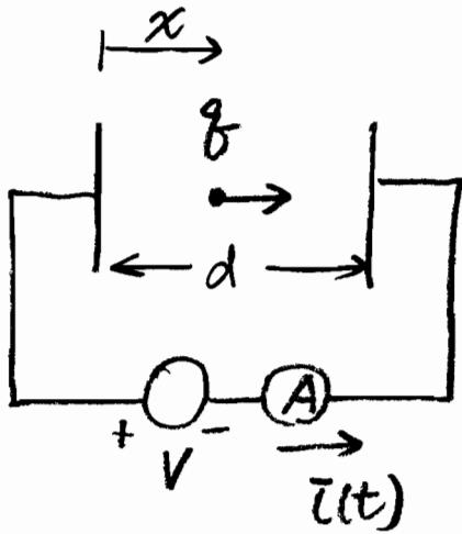
Current caused in the external circuit by a moving charge  $q$  in a parallel plate capacitor with a separation of  $d$  and voltage bias of  $V$ :
