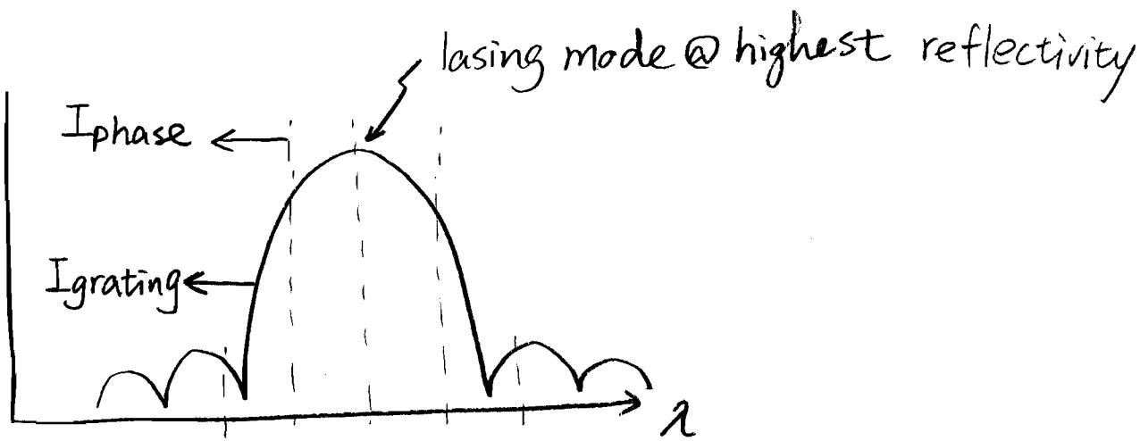
Increasing grating section current ( $I_{\text{grating}}$ ) moves reflectivity curve to shorter  $\lambda$  side, but does not change mode position much
