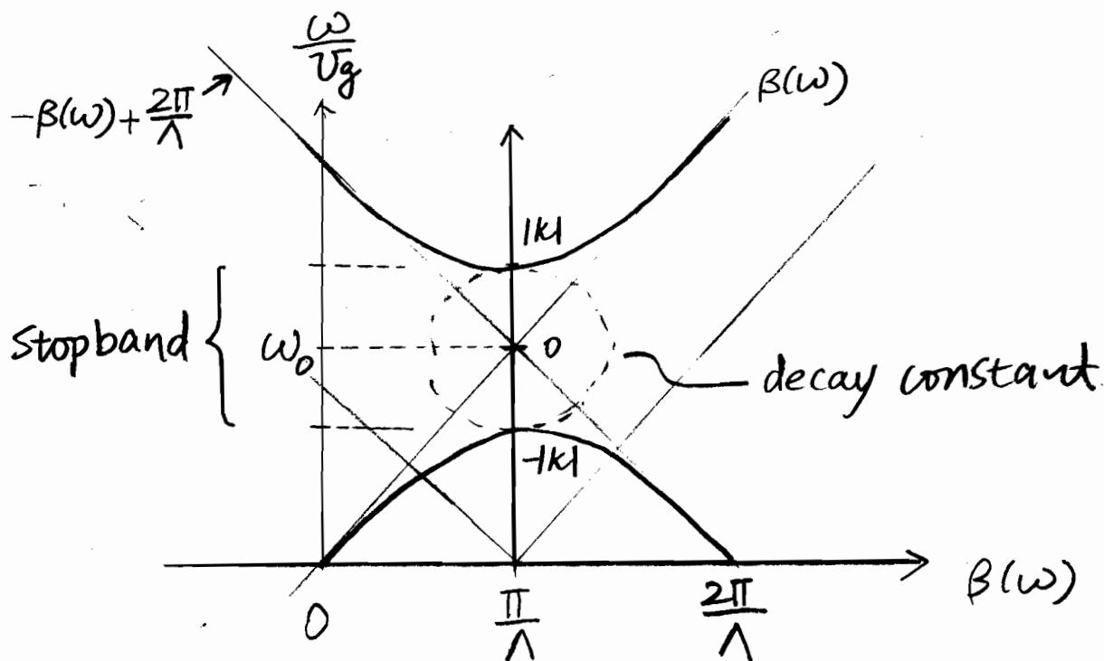
Expansion of  $\beta(\omega)$  around  $\omega_0 = 2\pi \frac{c}{\lambda g} = 2\pi \frac{c}{(2\lambda)}$
