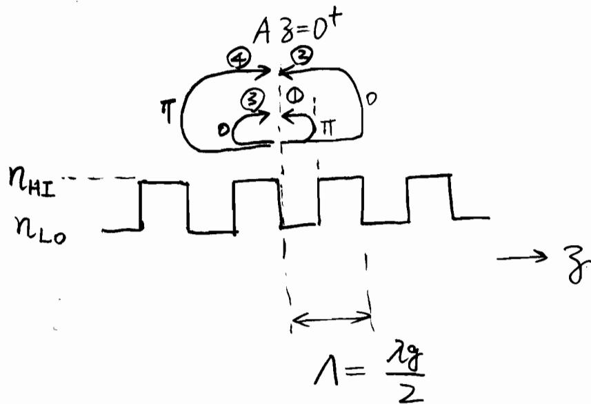
Phase shift for reflection is negative when going from high to low index
