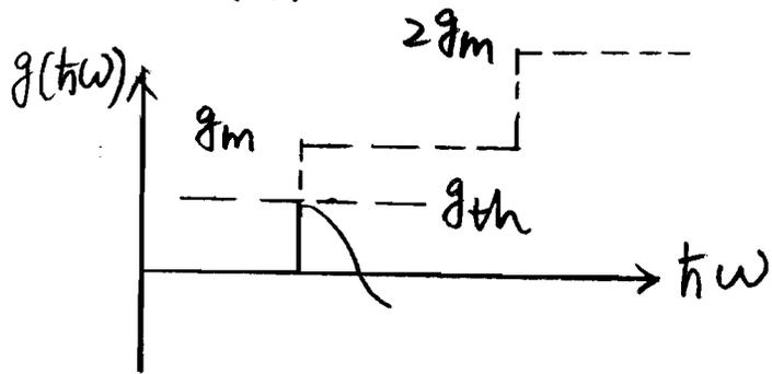
If  $g_{th} > g_m$ , we need to fill the first band until  $\Delta E_F > E_{h2}^{e2}(0)$ , resulting in high  $I_{th}$
