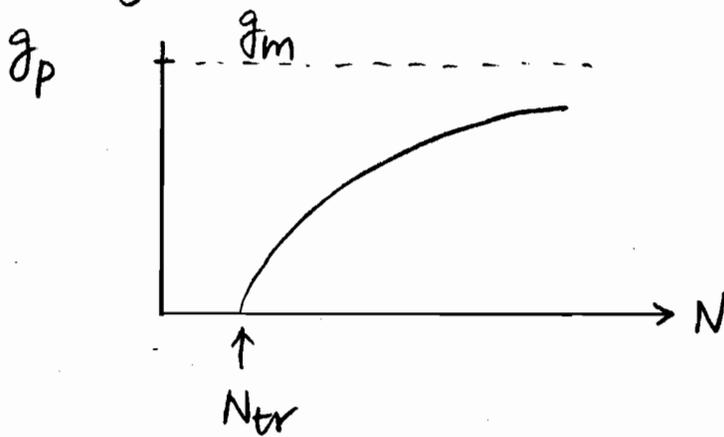
The gain-vs-current curve can be very well by a logarithmic shape:
