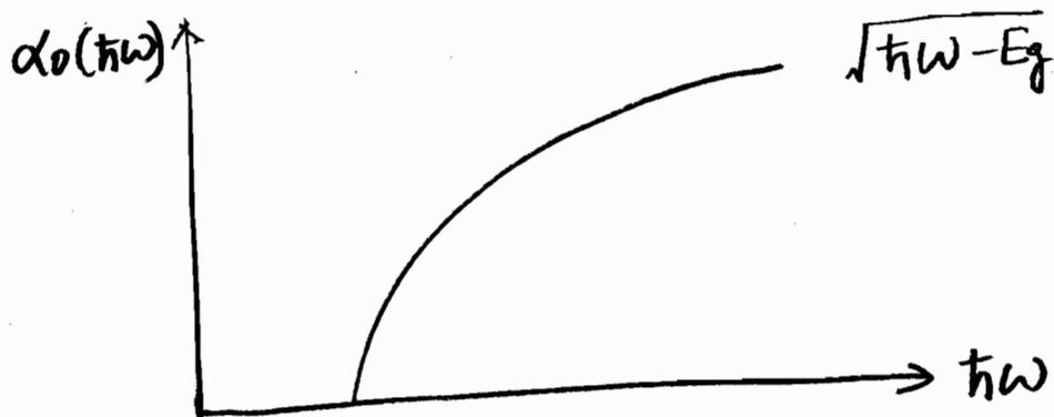
Spectral shape of  $\alpha_0(\hbar\omega) \rightarrow$  from joint optical DOS
