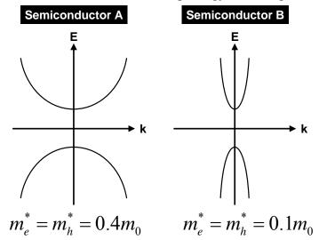
Both semiconductors have the same bandgap energy (1 eV) and the same optical matrix elements. This problem deals with the transparency carrier concentration,  $N_{tr}$ . This is the carrier concentration at which the *peak* gain is equal to zero. [Note that when peak gain is just equal to zero, the corresponding photon energy is equal to bandgap energy].
