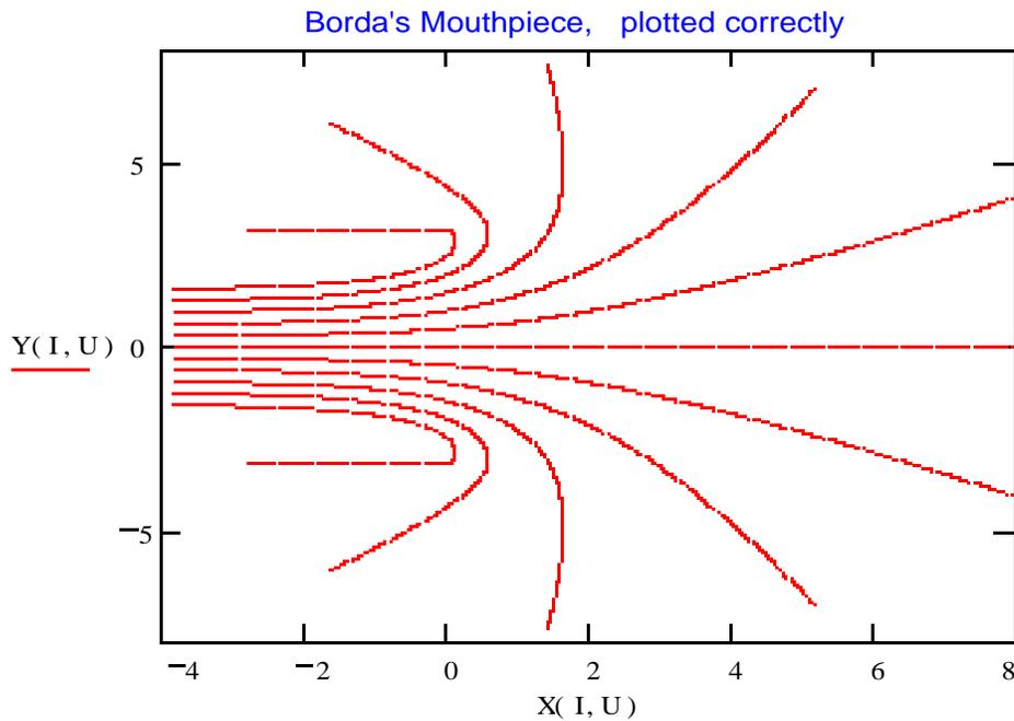
This plot shows the streamlines of a flow of an Ideal Fluid under high pressure escaping to the left through a channel with straight horizontal sides. Inside the channel, the flow's boundary is free, not touching the channel walls. Without -0, the flow along the outside of the lower channel wall is misplotted across the inner mouth of the channel and, though it does not show above, also as a short segment in the upper wall at its inside end. W. Kahan
