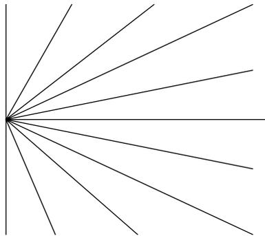
**The expected picture**, called “Borda’s Mouthpiece,” shows eleven streamlines of an ideal fluid flowing into a channel under such high pressure that the fluid’s surface tears free from the inside of the channel.
