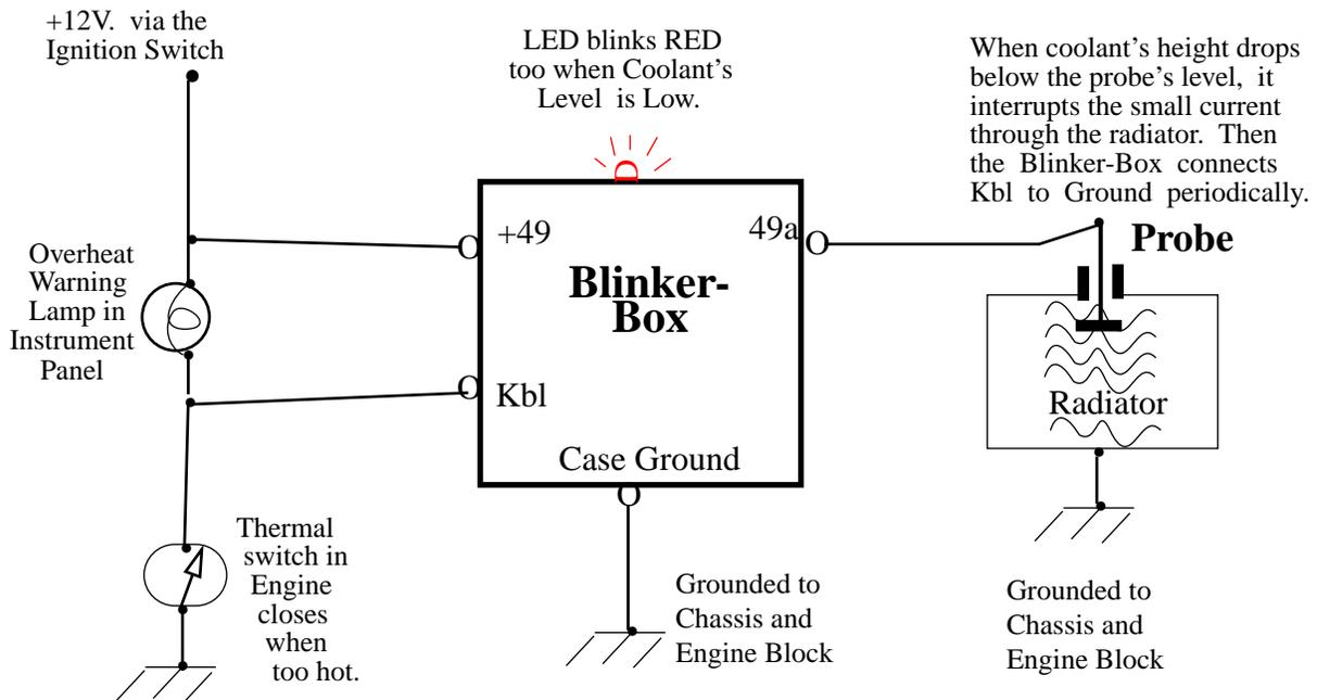
The engine's thermal switch closes when it gets too hot, thus turning on the warning lamp in the car's instrument panel. Before that can happen because of a loss of coolant, the Probe senses the coolant's lowered height in the radiator and signals the Blinker-Box to simulate a periodic closing of the thermal switch via the "Kbl" terminal, thus blinking the instrument panel's warning lamp.
