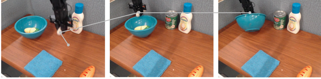
Figure 13: Grounding failure occurs when high level instruction is masked out. While the low level instruction “move the gripper left” correctly predicts the next reasonable action, masking out the context of the subtask “put the mushroom in the bowl” causes the policy to overshoot its trajectory.
