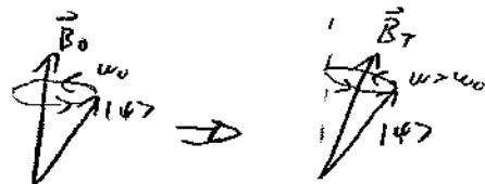
$\underline{\Rightarrow}$ , "Latitude" on Bloch Sphere DOES change, i.e., " $\theta$ " changes for  $|4\rangle = \cos \frac{\theta}{2} |0\rangle + e^{i\phi} \sin \frac{\theta}{2} |1\rangle$
