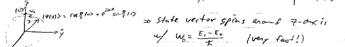
But, although  $H_0$  causes  $|\psi(t)\rangle$  to spin around  $\hat{z}$ -axis, it will never cause it to change "latitude" on Bloch sphere. i.e., No "spin-flips" or transitions. How do we do this?
