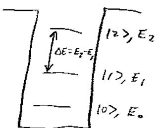
$\Rightarrow$  Shine light on atom at Frequency  $\omega = \frac{\Delta E}{\hbar} = \frac{E_2 - E_1}{\hbar}$
