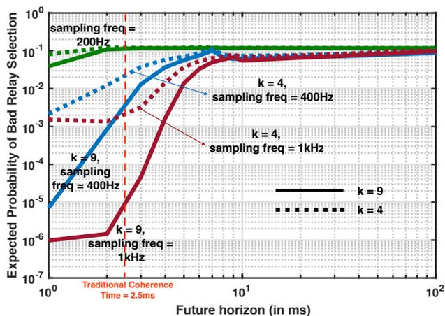
Fig. 6: Probability of best relay not being good enough for varying sampling frequency and future horizons. The model order is 3, the number of relays to choose from is  $k = 9$  (solid curves) and  $k = 4$  (dotted curves), nodes are moving in a random direction at speed 10m/s, nominal SNR is 5dB and the center frequency is  $f_c = 3$ GHz. The traditional coherence time for a radio moving at these parameters is 2.5ms (corresponding to moving  $\lambda/4$  at 10m/s) which is marked on the plot.
