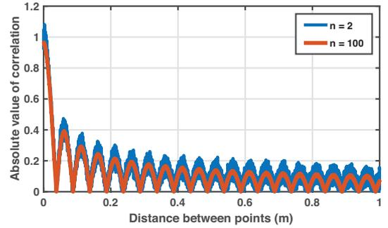
Fig. 2: Simulated absolute value of the cross-covariance of the fading process for  $f_c = 3\text{GHz}$ . The curves are exactly as predicted by Eq. 5 even for a small number of scatterers  $n = 2$ .
