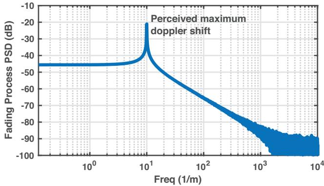
Fig. 3: One-sided PSD of the fading process for  $f_c = 3\text{GHz}$
