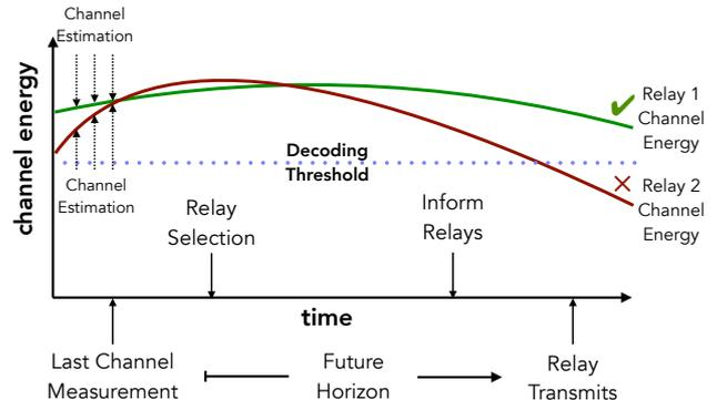
Fig. 1: After estimating channels, relays are selected and informed of their selection. During the time between channel estimation and the relays transmitting, the channels may change.
