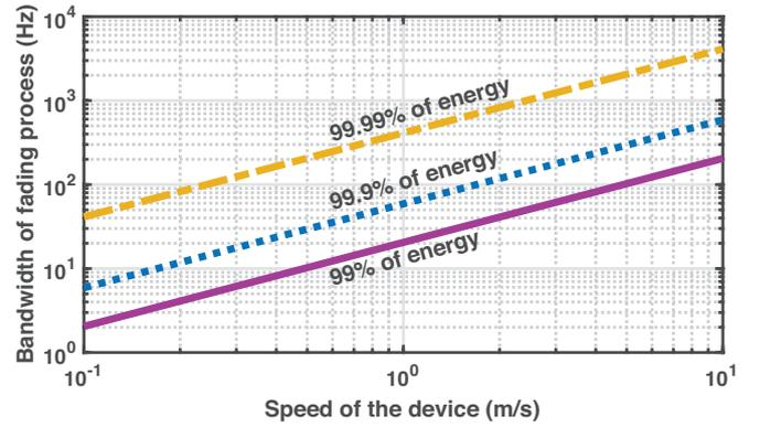
Fig. 4: Bandwidth around the center frequency which captures 99%, 99.9% and 99.99% of the energy of the fading process as a function of node speed
