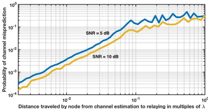
Fig. 5: The probability of channel quality misprediction as a function of how far the node has moved (at 10m/s) since the last channel measurement. This figure was obtained for a sampling frequency of 1kHz, and nominal SNRs 5 and 10dB.
