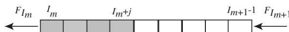
Fig. 10. In equilibrium n^{e,m} sections I_m, \dots, I_m + j of S^m are congested.
