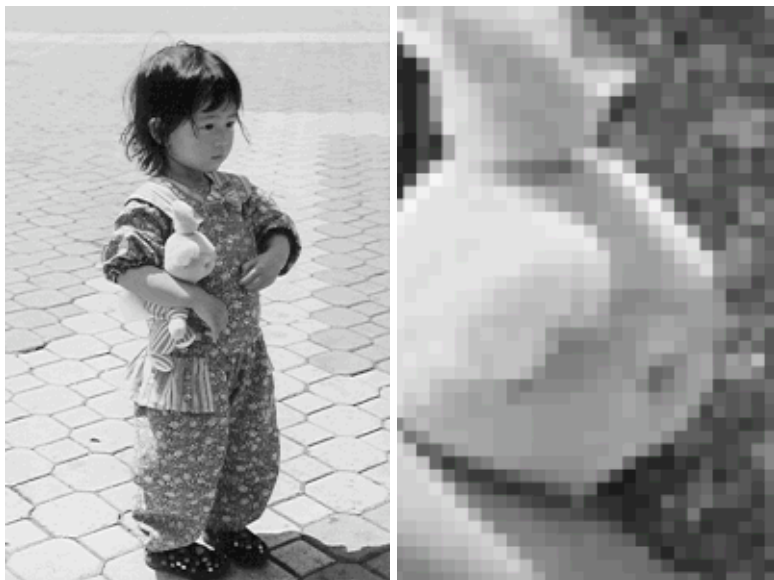
Figure 1.6: Grayscale image on the left, and its enlarged pixels on the right.
