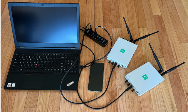
Figure 4: Our testbed uses an x86 laptop with two b210 SDRs acting as gNodeBs for two separate PLMNs and an Android phone with a programmable SIM.
