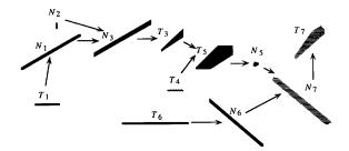
Fig. 11. Derivation of Thevenin and Norton representations for example circuit. The derivation follows the series-parallel decomposition.
