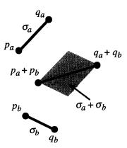
Fig. 6. Preservation on convexity by Minkowski sum. The segment connecting the sums of pairs of points from the arguments must lie within the parallelogram formed by summing the segments connecting the argument points.
