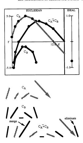
Fig. 9. Illustration of contour addition. Upper contours are summed by merging their segments in descending-slope order.
