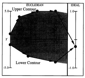
Fig. 5. Contour representation of a polygon. When a polygon includes ideal points, the minimum and maximum points give the slope of the rightmost lower and upper edges.
