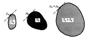
Fig. 7. Addition of convex sets. The boundary of the sum can be formed by sweeping around the arguments with a pair of parallel tangents.
