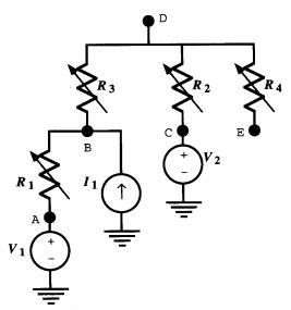
Fig. 12. Representation of example circuit as a grounded tree. By replicating the ground node, the circuit attains a tree structure.
