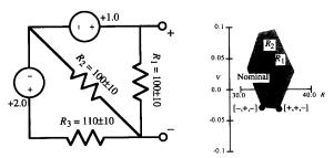
Fig. 1. Example of variable resistor circuit. The range of possible Thevenin equivalent circuits forms a convex polygon.
