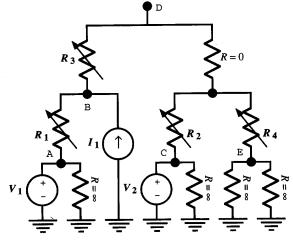
Fig. 13. Transformation of circuit into binary tree. High degree nodes are split and connected by perfect conductors, while low degree nodes are connected to ground by insulators.
