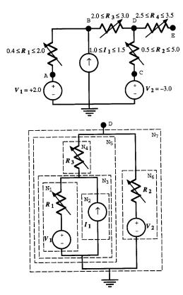
Fig. 10. Circuit and its series-parallel decomposition. This decomposition characterizes the circuit at D with respect to ground.
