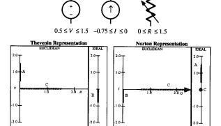
Fig. 4. Variable circuit elements and their representations. Each is represented by a segment in both the Thevenin and Norton half-planes.
