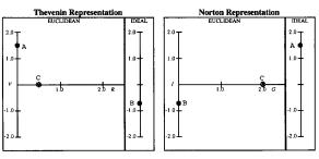
Fig. 2. Geometric representations of fixed circuit elements. Each element is represented by a point in the Thevenin and Norton half-planes.
