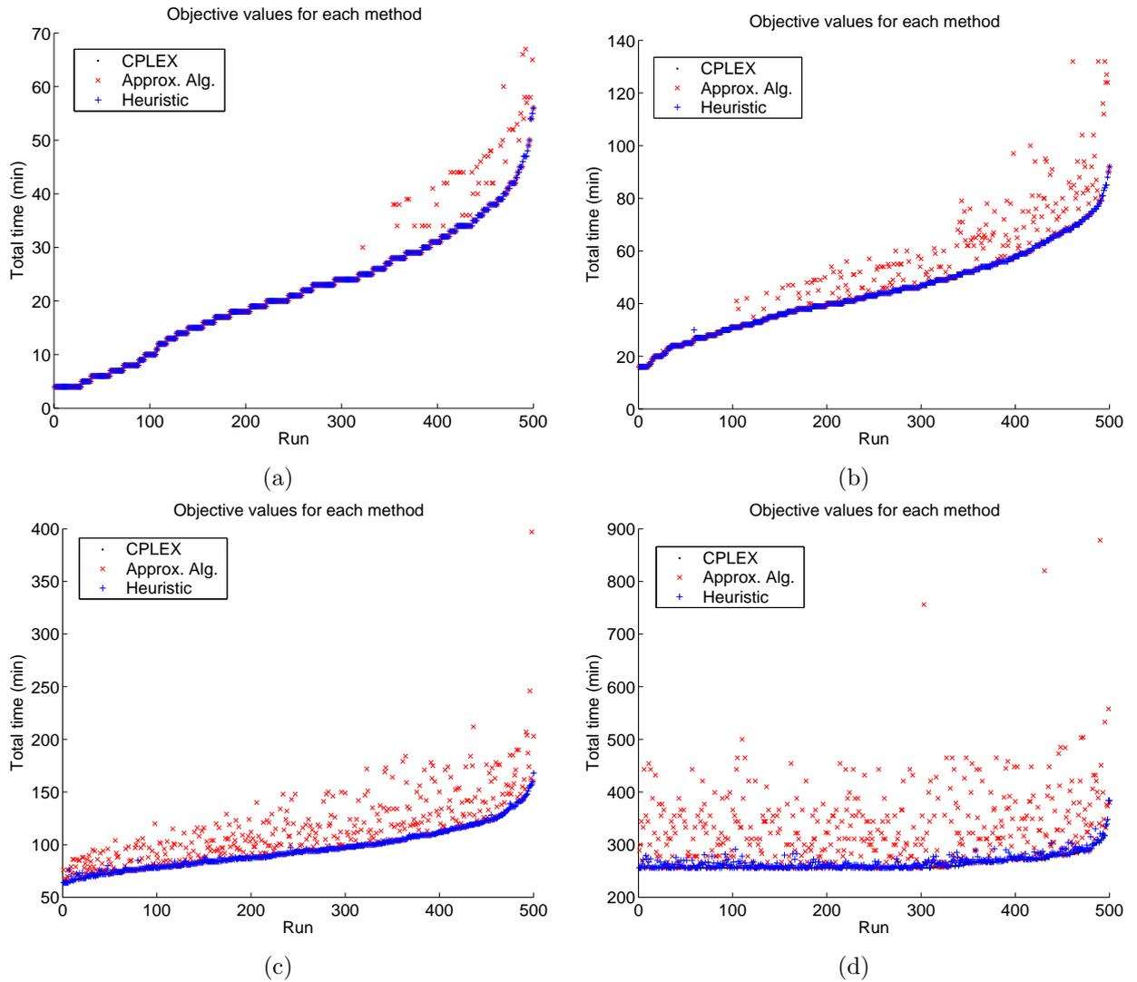
Figure 7. Objective values (i.e. sum of arrival times) for each of 500 runs for CPLEX, approximation, and heuristic algorithms for required spacing  $\Delta = 2$ , holding pattern time  $T=10$ , and different numbers of aircraft  $N$ .  $N =$  (a) 2; (b) 4; (c) 8; (d) 16. The runs are sorted by increasing CPLEX objective value, but a given x-value shows results of each algorithm on the same parameter values.
