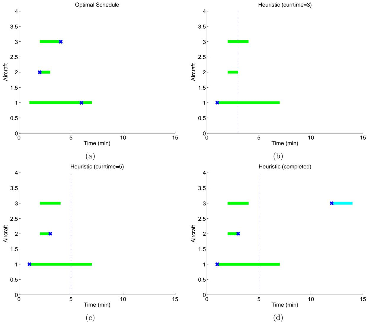
**Figure 3.** (a) Optimal scheduling of three aircraft with landing intervals marked as horizontal line segments and landing times marked by x's. (b) Heuristic algorithm after landing first aircraft. (c) Heuristic algorithm after landing second aircraft. (d) Heuristic algorithm at completion, having placed third aircraft on holding pattern.
