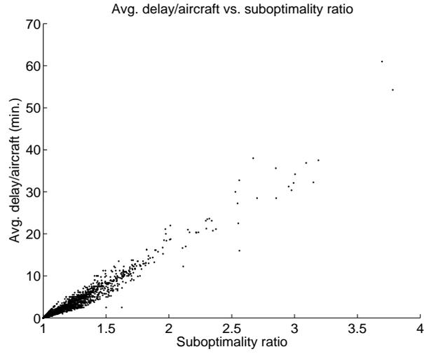
Figure 10. Average added delay per aircraft versus suboptimality ratio for all simulated runs.
