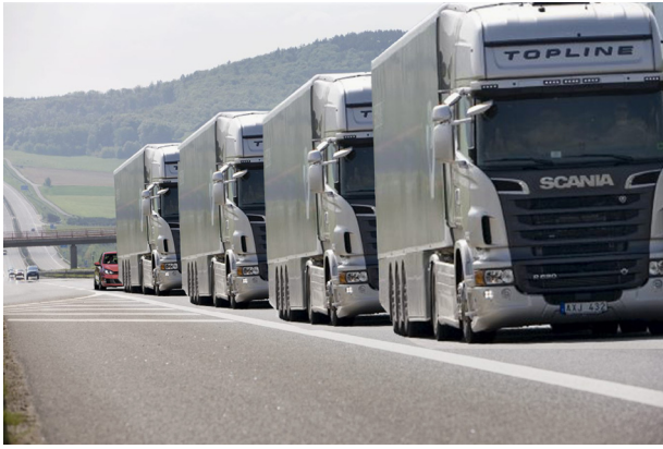
Fig. 1. HDVs traveling in a platoon can achieve significant fuel reduction.
