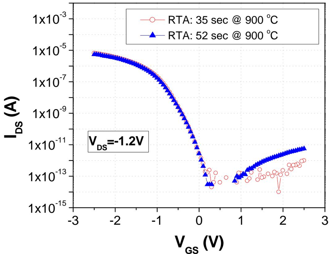
Figure 5.4: Effect of RTA conditions on the  $I_{DS}$ - $V_{GS}$  characteristics of the p-channel GSS FinFET NVM cell design shown in Figure 5.1(a). ( $L_g=0.5\mu\text{m}$ ,  $W=0.1\mu\text{m}$ ,  $V_{DS}=-1.2V$ ).
