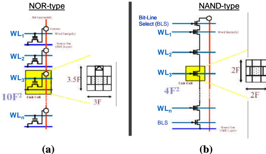
Figure 1.7: Predominant NVM array architectures [1.10]: (a) Common-Source NOR-type array architecture (mainly used for embedded applications). (b) NAND-type array architecture (mainly used for mass storage applications).
