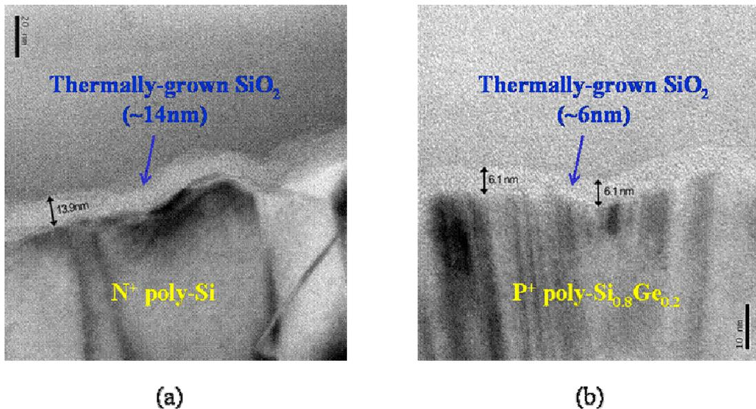
Figure 4.6: Cross-sectional TEM images that show the thickness of the control oxide film grown along the sidewalls of the in-situ doped (a)  $n^+$  Poly-Si and (b)  $p^+$  Poly-Si<sub>0.8</sub>Ge<sub>0.2</sub> film.
