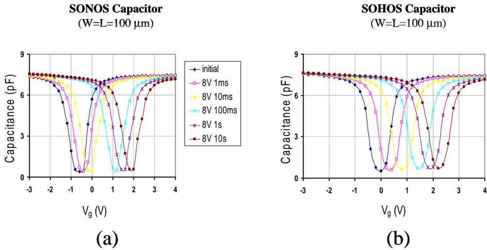
Figure 2.5: Capacitance vs. Voltage (C-V) Measurements (before and after application of various 8-volt programming pulses at the gate) of capacitors containing (a) the SONOS structure, and (b) the SOHOS structure.
