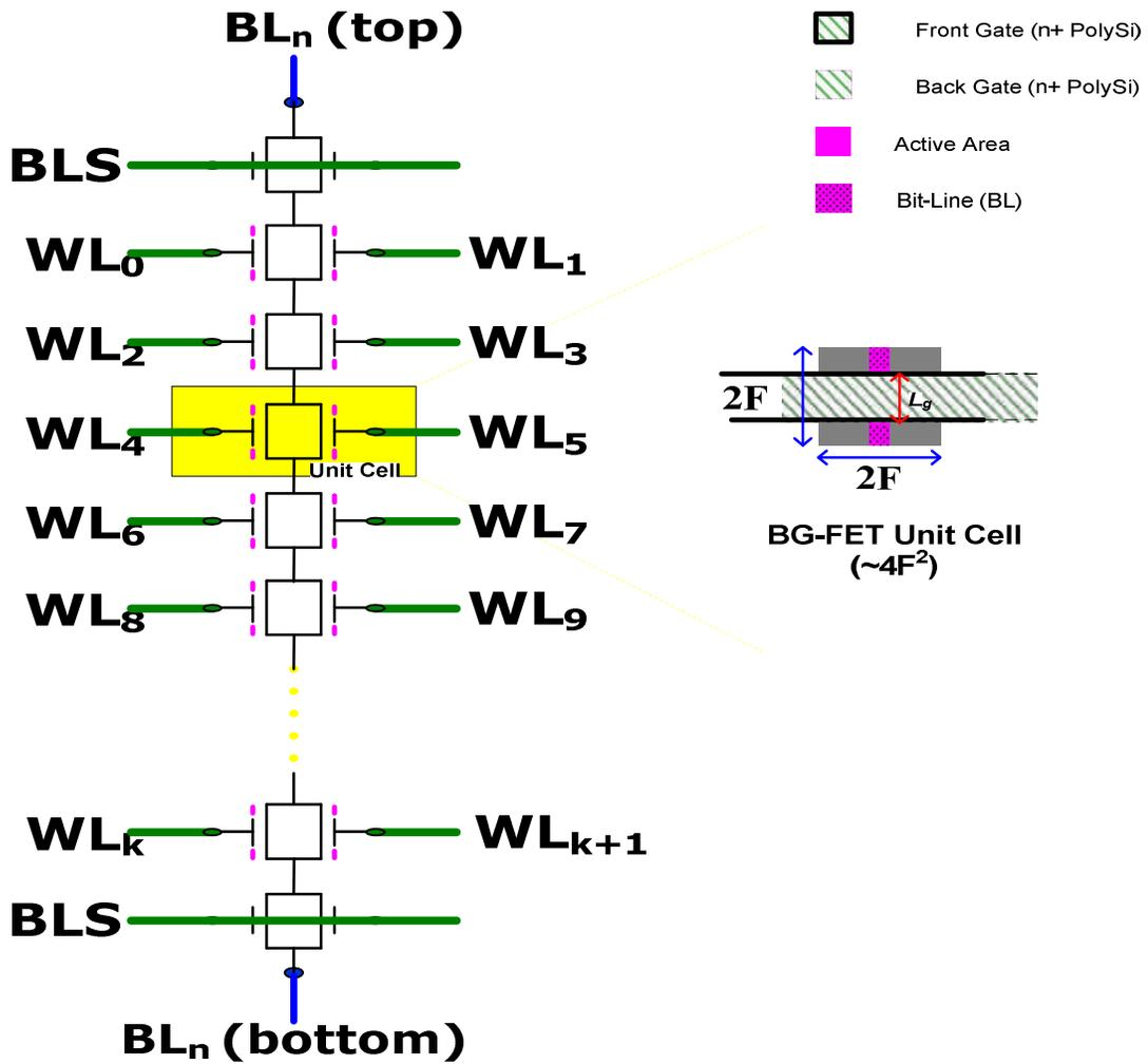
Figure 6.19: Unit cell layout of a BG-FET cell design within a NAND-type Array Architecture.
