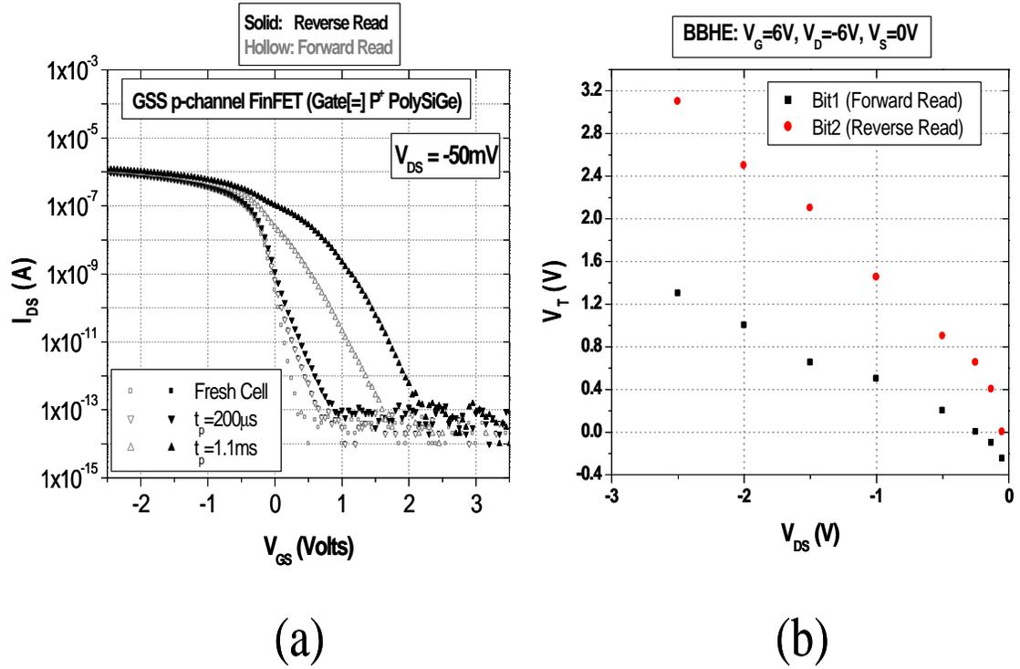
Figure 5.7: Measured  $I_{DS}$ - $V_{GS}$  curves of a p-channel GSS FinFET NVM cell (Figure 5.1a) before and after various BBHE ( $V_{GS}=6V$ ,  $V_{DS}=-6V$ ) programming pulses ( $t_p$ ) were applied to the structure ( $L_g=0.5\mu m$ ,  $W=100nm$ ,  $V_{DS}=-50mV$ ). (b)  $V_T$  of both bits as a function of  $V_{DS}$ .
