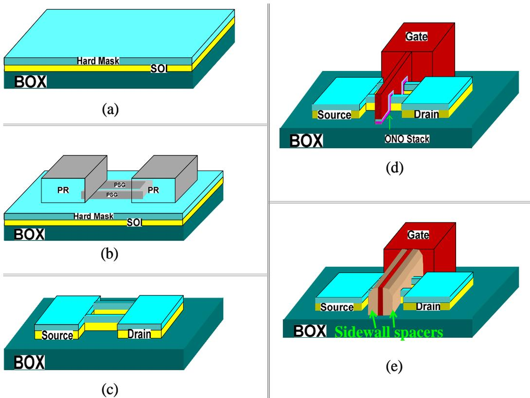
Figure 3.9: Process flow used to fabricate the dual-bit SONOS FinFET NVM cell.
