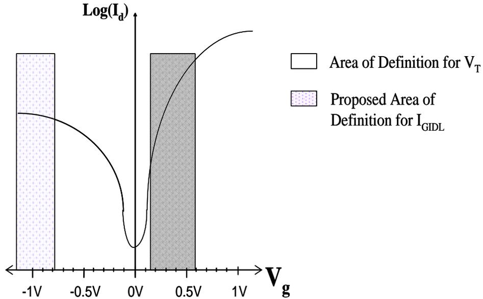
Figure 2.9: Illustrations that show the regions of the  $I_{DS}$ - $V_{GS}$  curve where the transistor's threshold voltage ( $V_T$ ) and 'saturated' GIDL current [2.12] would normally occur.
