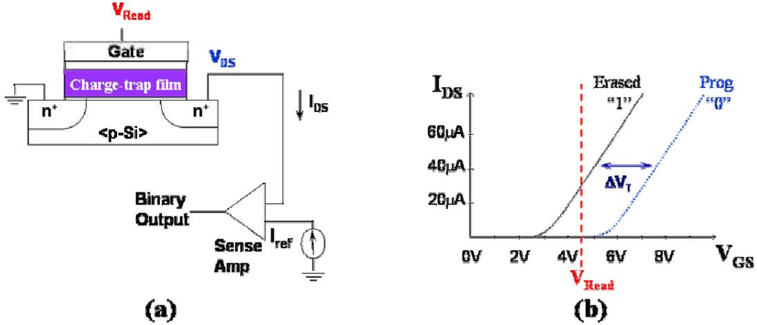
Figure 1.3: Read operation in a NVM cell: (a) Measurement setup. (b) A measure of the cell’s on-state  $I_{DS}$  current (at a specific gate voltage, ‘ $V_{Read}$ ’, and drain-to-source voltage, ‘ $V_{DS}$ ’) permits identification of the binary state of the NVM cell.
