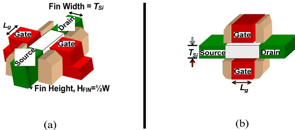
Figure 6.5: Independent Gate DG-FET designs: (a) 3D Multiple Independent Gate FET (MIGFET) design [6.20]. (b) Planar Back-Gated FET (BG-FET) design [6.5].
