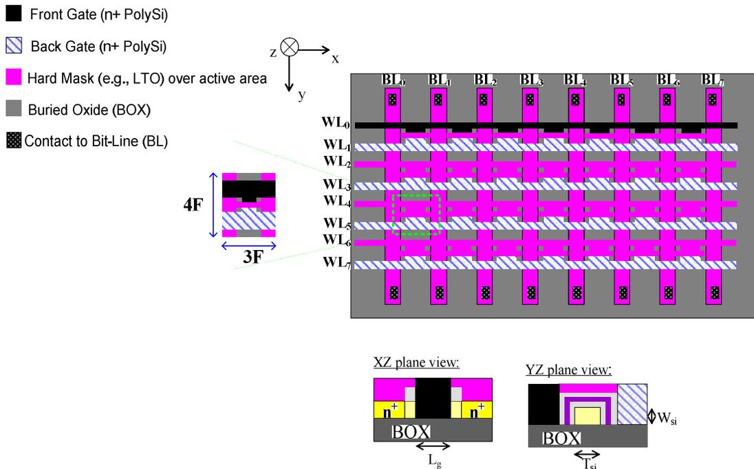
Figure 6.16: NOR-type array architecture layout (based on SOI technology) that utilizes the MIGFET structure as its unit cell. The placement of both word-lines on the side (instead of on top) of the active area and their required isolation significantly increases the size of its unit cell.
