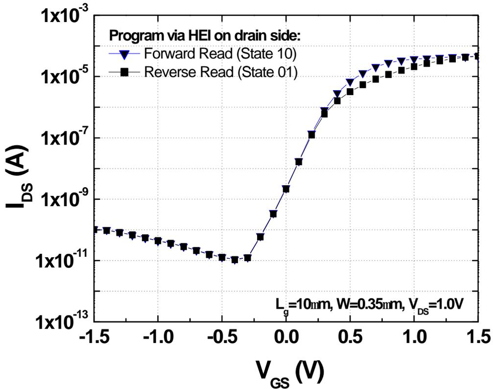
Figure 4.9: (a) Measured  $I_{DS}$ - $V_{GS}$  characteristics of a dual-bit GSS n-channel FinFET NVM cell ( $n^+$  Poly-Si gate) with gate-overlapped source/drain regions ( $L_g=10\mu m$ ,  $W=1\mu m$ ,  $V_{DS}=1.0V$ ), showing a negligible change in  $V_T$  (and no change in GIDL current) when charge is stored on the drain-side bit via HEI (programming conditions:  $V_G = 7V$ ,  $V_{DS} = 7V$ , 10ms).
