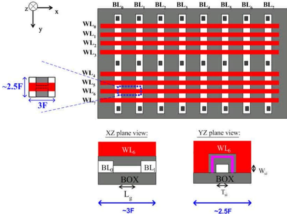
Figure 3.16: NOR-type array architecture layout (based on SOI technology) that utilizes the SONOS FinFET structure as its unit cell.
