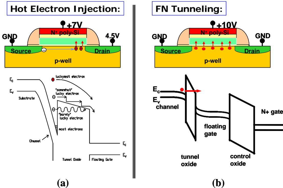
Figure 1.4: Predominant programming mechanisms: (a) Hot Electron Injection (HEI). (b) Fowler-Nordheim (FN) Tunneling.
