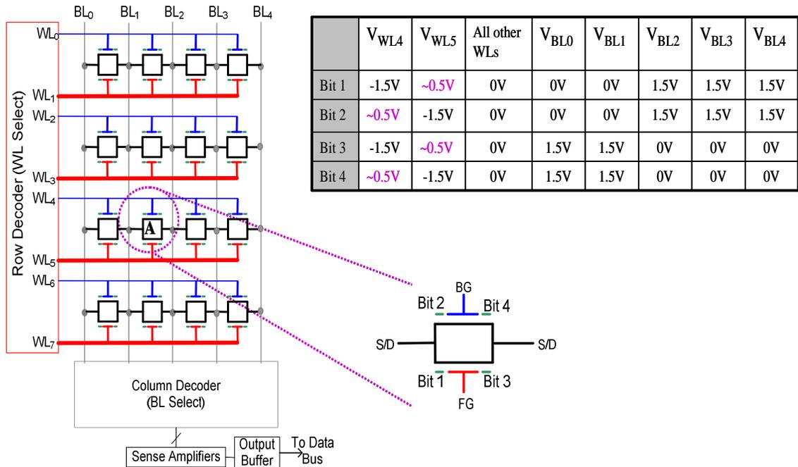
Figure 6.15: Schematic circuit diagram of 4-bit DG-FET NVM cells arranged in a NOR array architecture. Bias voltages used to read each bit of Cell ‘A’ are indicated in the Table.
