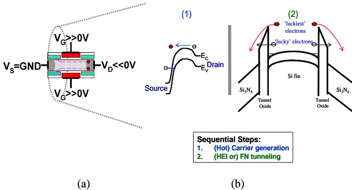
Figure 5.6: Programming disturbance of the BBHE programming method: (a) Bias conditions. (b) Energy band diagrams used to describe the injection of electrons in the complementary bit (next to the Source electrode).
