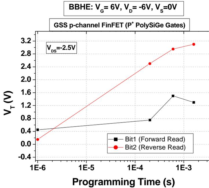
Figure 5.8: Measured BBHE programming characteristics ( $V_{DS}=-2.5V$ ) of a p-channel GSS FinFET NVM cell with p+ PolySi gates. ( $L_g=0.5\mu m$ ,  $W=100nm$ ).
