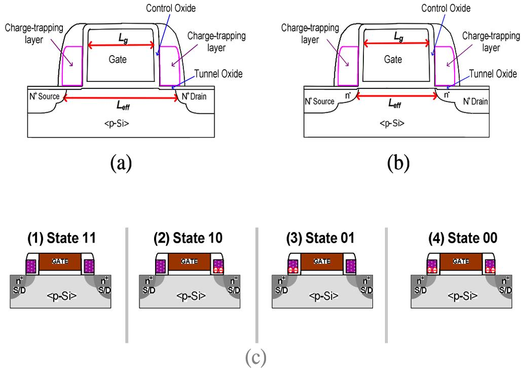
Figure 7.1: 2D schematic cross-sections of (a) a gate-underlapped ( $L_{eff} > L_g$ ), and (b) a gate-overlapped ( $L_{eff} \sim L_g$ ) NVM cell structure with charge storage sites located at the gate sidewalls. (c) Definition of the 4 charge-storage states of this dual-bit cell.
