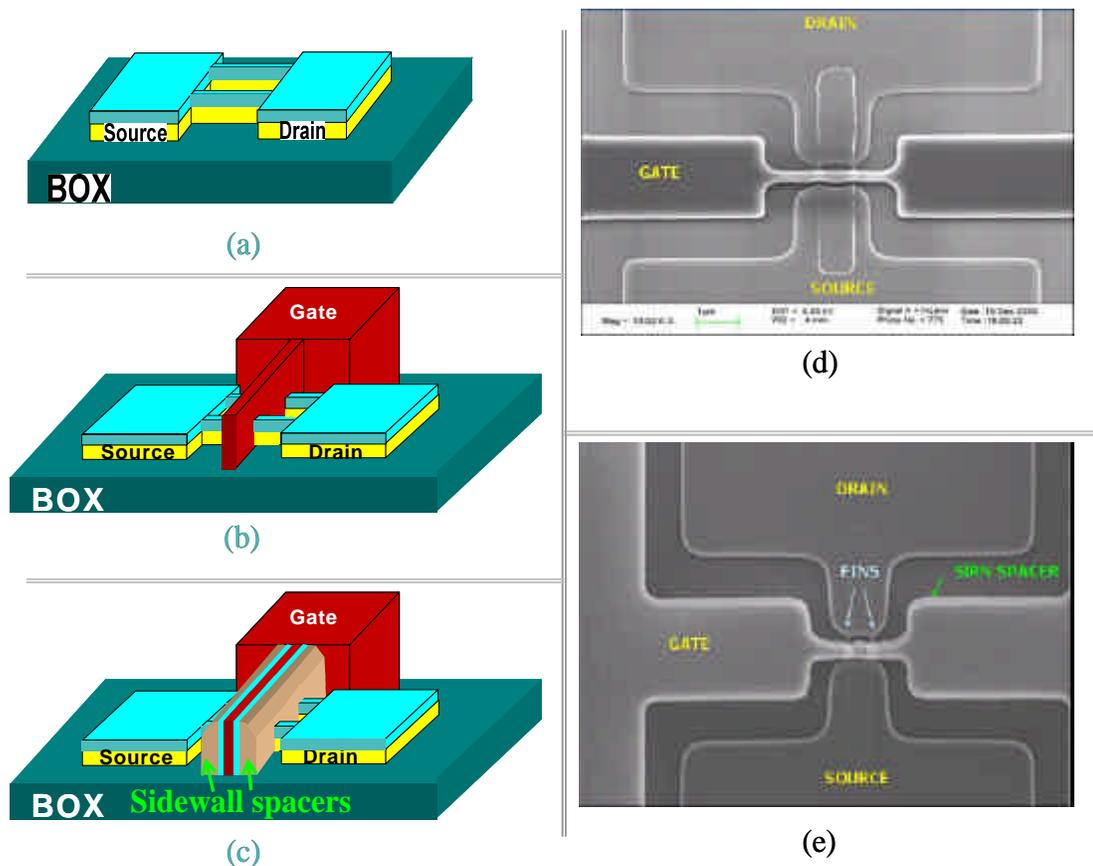
Figure 4.5: (a-c) Process flow used to fabricate gate-sidewall storage (GSS) FinFET NVM cells –Gate Area, Spacer Definition. (d-e) SEMs of a fabricated cell after completion of processing steps (b) and (c), respectively.
