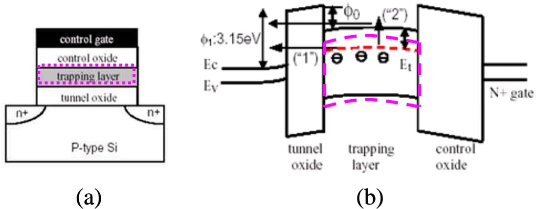
Figure 2.3: (a) Proposed structure, which utilizes a charge-trapping material with a larger electron affinity than  $\text{Si}_3\text{N}_4$ . (b) Energy band diagram, showing the improvement in charge retention with the proposed structure (due to its larger conductivity band offset,  $\phi_0$ ).
