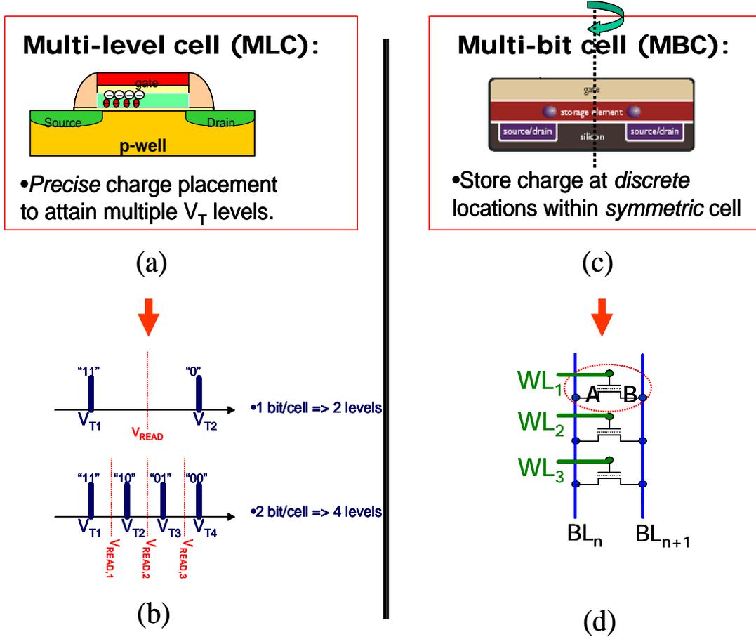
Figure 6.1: In the MLC design (a), different  $V_T$  levels, one for each binary state (b), are defined to store multiple bits in every cell. The MBC design (c) utilizes the cell's symmetry to access the information stored in either side ("A" or "B") of the cell (d).
