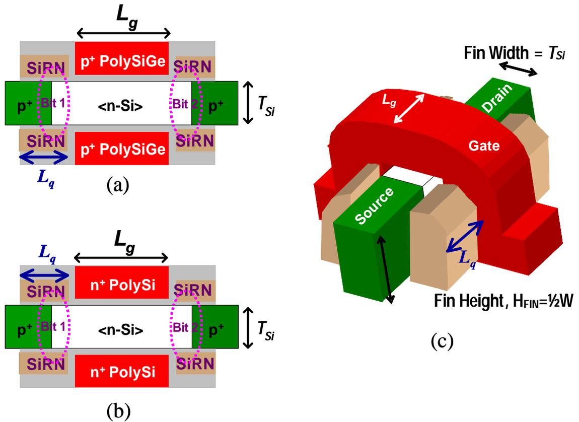
Figure 5.1: (a-b) Schematics of the two p-channel NVM cell designs studied in this chapter. (c) Isometric view of a dual-bit GSS FinFET NVM cell [5.13].
