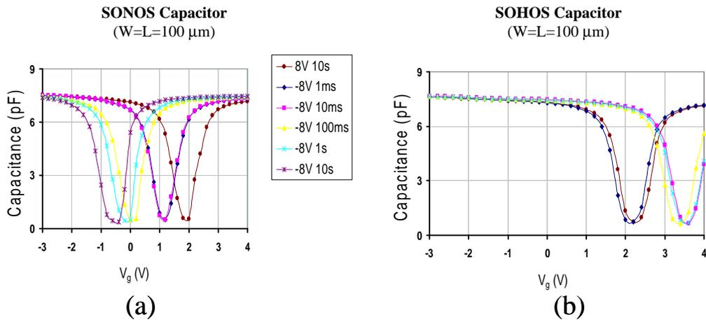
Figure 2.7: C-V Measurements (before and after application of various erasing pulses at the gate of a programmed structure) of capacitors containing (a) the SONOS structure, and (b) the SOHOS structure.
