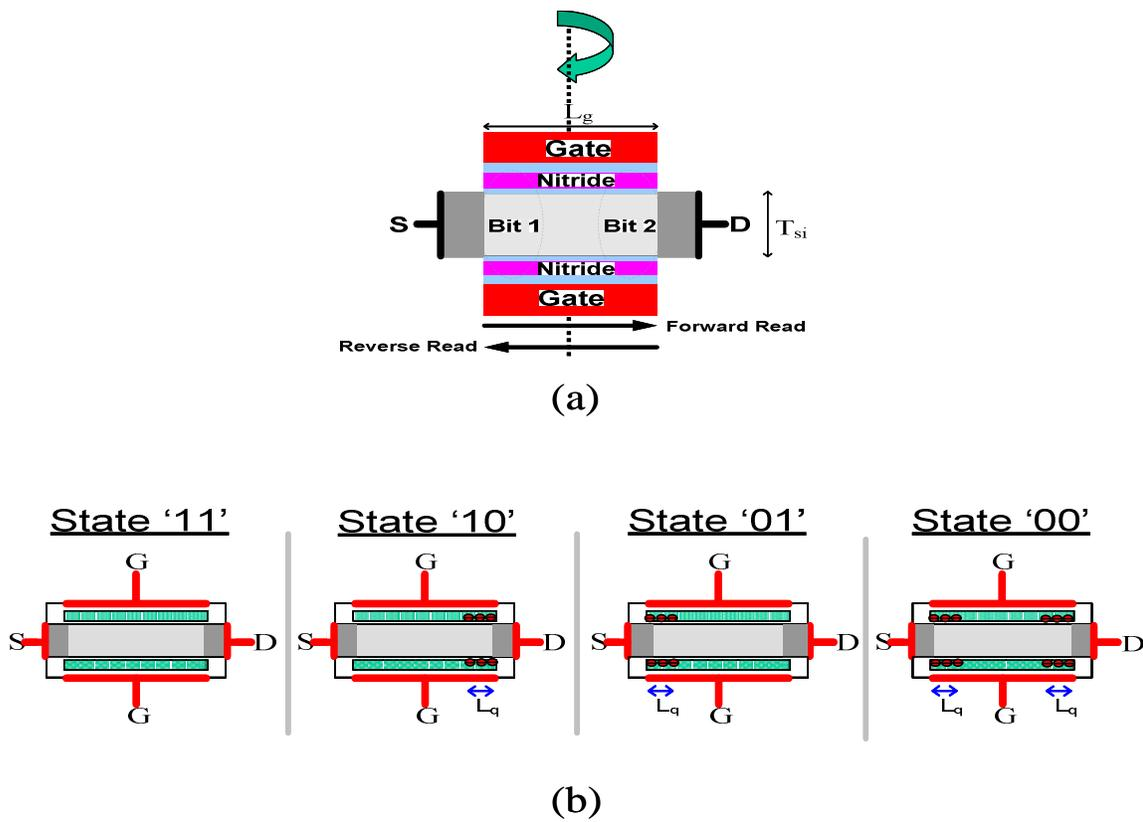
Figure 3.2: (a) the symmetry of the SONOS FinFET NVM cell (with respect to the S/D electrodes) allows for dual-bit operation. (b) Definition of the 4 binary states of this dual-bit NVM SONOS cell.
