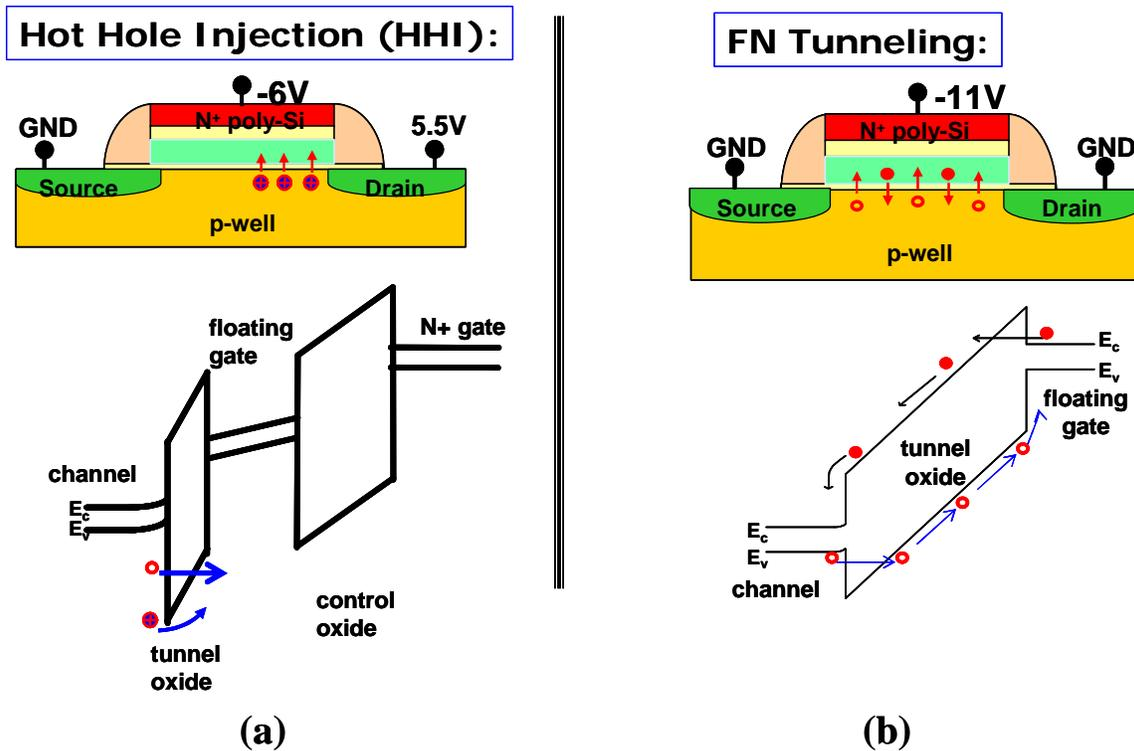
Figure 1.5: Predominant erase mechanisms: (a) Hot Hole Injection (HHI). (b) Fowler-Nordheim (FN) Tunneling.
