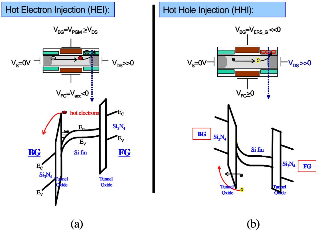
Figure 6.8: Each bit of the 4-bit DG-FET structure can be selectively programmed and erased via the conventional (a) Hot Electron Injection, and (b) Hot Hole Injection methods, respectively.
