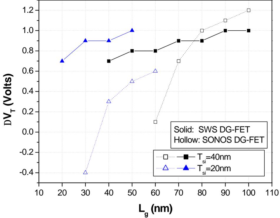
Figure 6.12: Simulated threshold voltage shift ( $\Delta V_T$ ) due to charge storage at Bit 1 as a function of the cell's gate length ( $L_g$ ). As can be seen, the 4-bit SWS DG-FET structure is more scalable than the 4-bit SONOS DG-FET.
