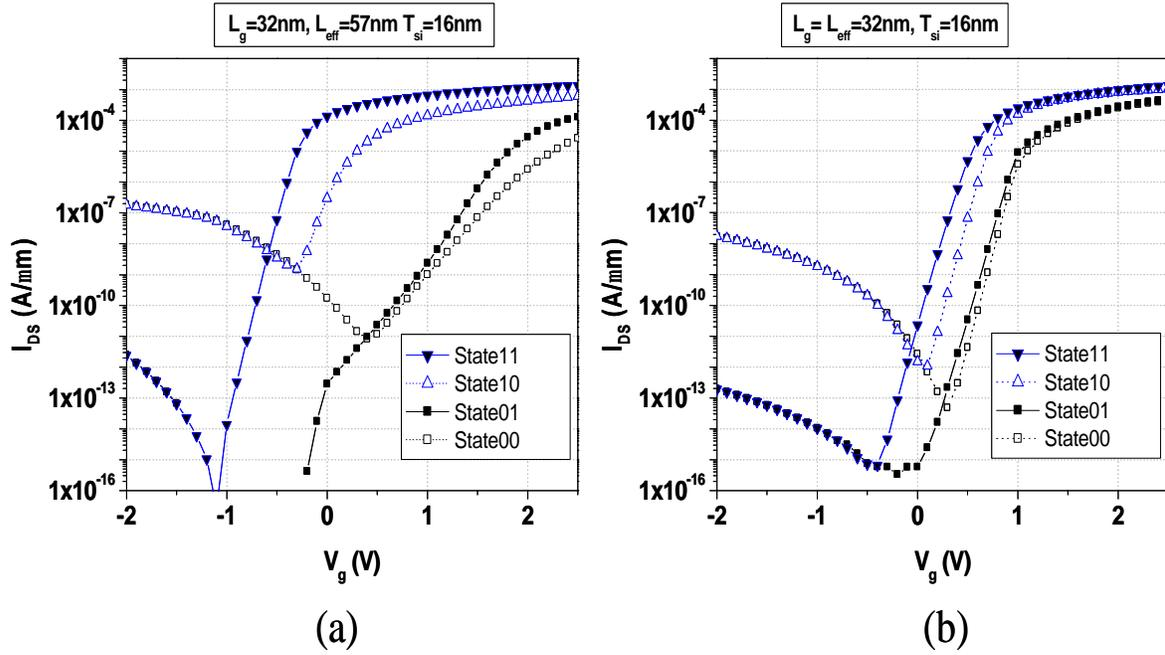
Figure 4.3: Simulated  $I_{DS}$ - $V_{GS}$  ( $V_{DS}=1.5\text{V}$ ) characteristics for each state of a gate-sidewall-storage FinFET NVM cell with (a) gate-underlapped source/drain regions and (b) gate-overlapped source/drain regions
