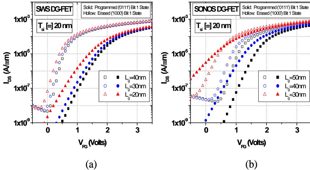
Figure 6.11: Simulated  $I_{DS}$  vs.  $V_{FG}$  characteristics for the 2 binary Bit 1 states with smallest  $V_T$  separation ( $\Delta V_T$ ) of a (a) SWS DG-FET, and (b) SONOS DG-FET structure (for various gate lengths ( $L_g$ ) and for a specific silicon body thickness ( $T_{si}=20\text{nm}$ )).
