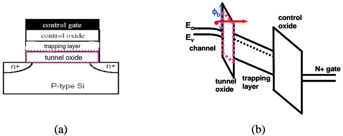
Figure 2.4: (a) Proposed charge-trapping NVM structure, which utilizes a high- $\kappa$  dielectric as the tunnel oxide. (b) Energy band diagram, showing the improvement in programming speed (as a result of the smaller  $\phi_b$  with the use of the new tunnel oxide film).
