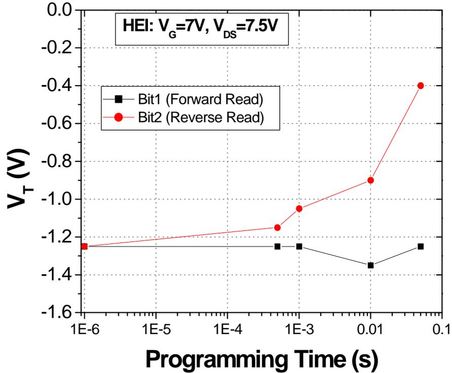
Figure 4.8: Measured HEI programming characteristics of an n-channel GSS FinFET NVM cell ( $p^+$  Poly-Si<sub>0.8</sub>Ge<sub>0.2</sub> gate). ( $L_g=240\text{nm}$ ,  $W=100\text{nm}$ ,  $T_{si}=75\text{nm}$ ,  $V_{DS}=1.2\text{V}$ ).
