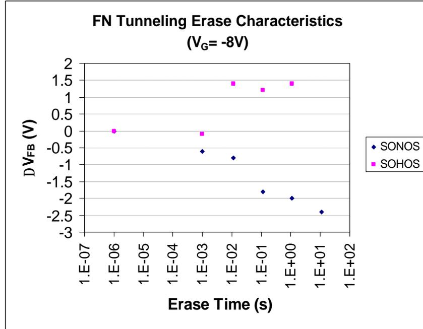
Figure 2.8: Erase Characteristics: Flat-band voltage shift ( $\Delta V_{FB}$ ) vs. erase time (at  $V_G = -8V$ ) for both SONOS, SOHOS devices.
