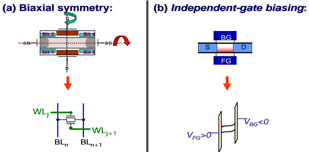
Figure 6.6: The operation of a 4-bit DG-FET NVM cell is based on two concepts: (a) Biaxial symmetry, which allows independent access of each charge storage site, and (b) Independent-gate biasing, which allows the masking of information stored at the unselected gate (e.g. the BG) as necessary.
