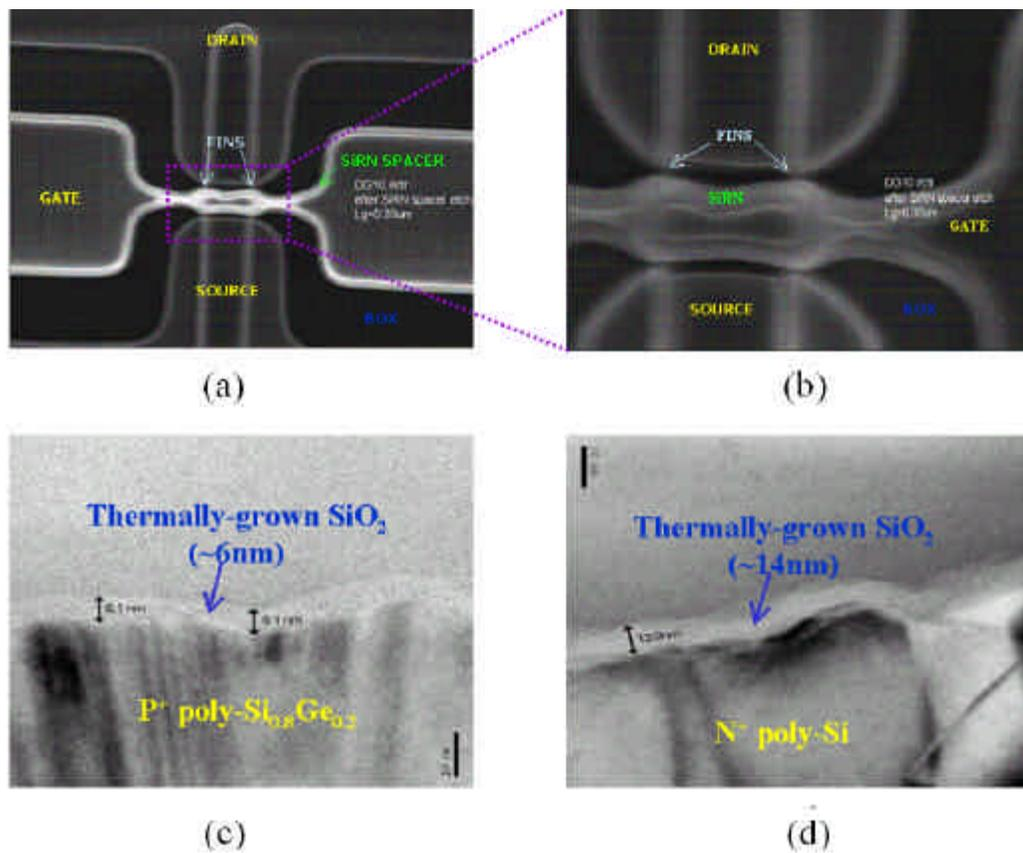
Figure 5.3: (a-b) SEM view of a p-channel GSS FinFET NVM cell after silicon-rich nitride (SiRN) spacer definition. The cross-sectional TEM images in (c-d) show the thickness of the control oxide grown along the sidewalls of the in-situ doped (c)  $\text{P}^+$  poly- $\text{Si}_{0.8}\text{Ge}_{0.2}$  and (d)  $\text{N}^+$  poly-Si gate films (respectively).
