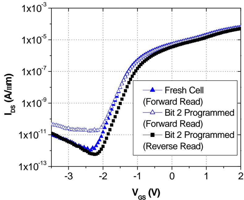
Figure 4.7: Measured  $I_{DS}$ - $V_{GS}$  curves of an n-channel GSS FinFET NVM cell ( $p^+$  Poly- $Si_{0.8}Ge_{0.2}$  gate) before and after Bit2 was programmed via HEI ( $V_{GS}=7V$ ,  $V_{DS}=7.5V$ ,  $500\mu s$ ). ( $L_g=240nm$ ,  $W=100nm$ ,  $T_{si}=75nm$ ,  $V_{DS}=1.2V$ ).
