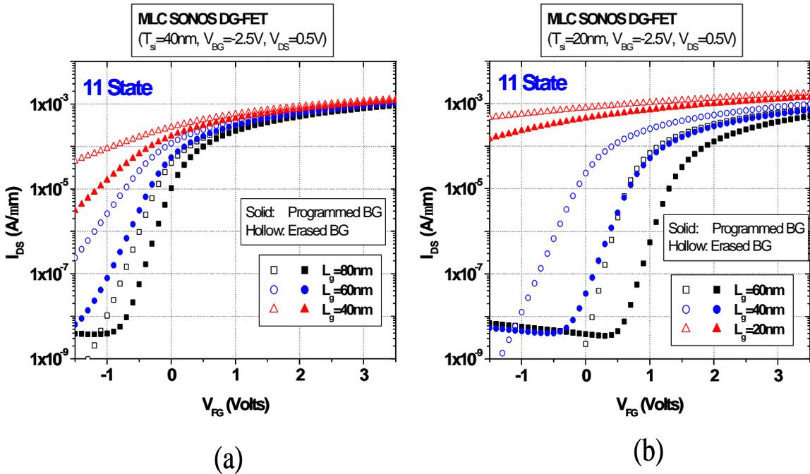
Figure 6.14: Simulated  $I_{DS}$  vs.  $V_{FG}$  characteristics ( $V_{BG}=-2.5\text{V}$ ,  $V_{DS}=0.5\text{V}$ ) for the erased state of a MLC SONOS DE\_FET cell, with the BG either fully erased or programmed to the highest  $V_T$  level, for various  $L_g$ . (a)  $T_{si}=40\text{nm}$ . (b)  $T_{si}=20\text{nm}$ .
