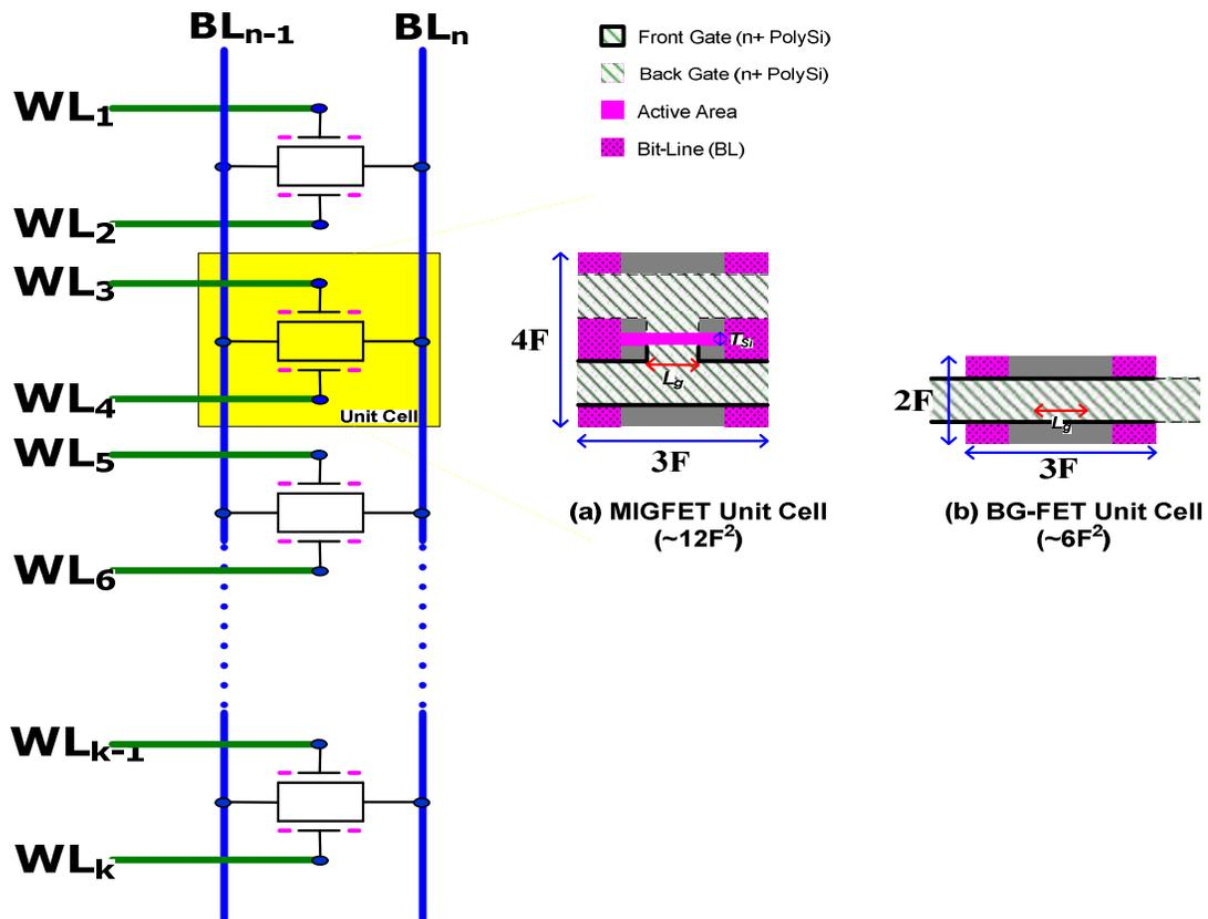
Figure 6.17: Unit cell layout of (a) a MIGFET cell design, and (b) a planar BG-FET cell design within a NOR-type array architecture. The use of a planar BG-FET as a 4-bit DG-FET cell significantly reduces the size of each unit cell ( $\sim 6F^2$ ) with this architecture [6.6].
