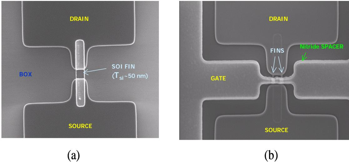
Figure 3.10: Scanning Electron Micrograph (SEM) images of the FinFET SONOS NVM cell after (a) Active area formation, and (b) Nitride spacer formation.
