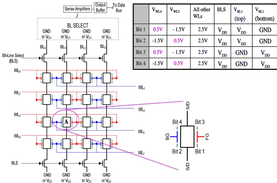
Figure 6.18: Schematic circuit diagram of 4-bit DG-FET NVM cells arranged in a NAND array architecture. Bias voltages used to read each bit of Cell 'A' are indicated in the Table.
