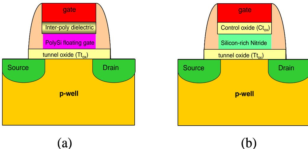
Figure 2.1: (a) Floating-gate versus (b) charge-trap-based (e.g., SONOS) NVM cell structures.
