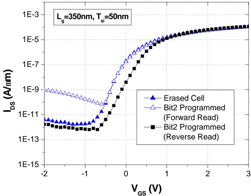
Figure 3.11: Measured  $I_{DS}$ - $V_{GS}$  characteristics ( $V_{DS}=1.5\text{V}$ ) of a SONOS FinFET cell before and after Bit 2 was programmed via HEI ( $V_{GS}=7.5\text{V}$ ,  $V_{DS}=8.0\text{V}$ ,  $80\mu\text{s}$ ).
