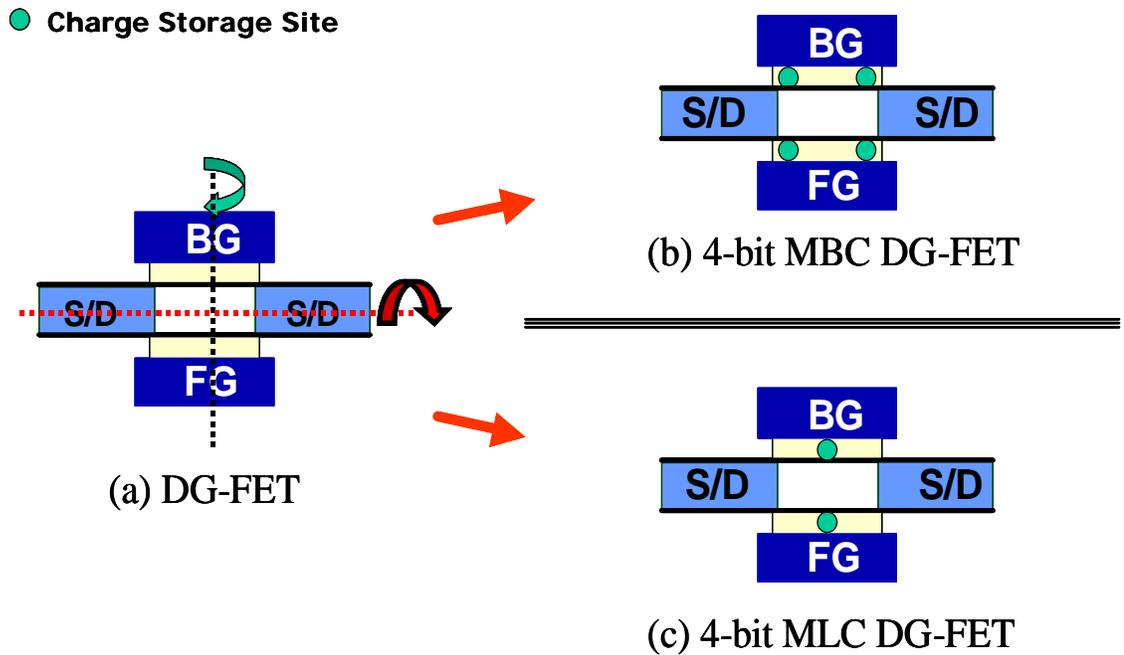
Figure 6.3: 4-bit DG-FET NVM Cell Designs: (a) The enhanced symmetry of a DG-FET structure permits its operation as either (b) a MBC DG-FET design (with 4 charge storage sites) or (c) a MLC DG-FET design (with 2 charge storage sites).
