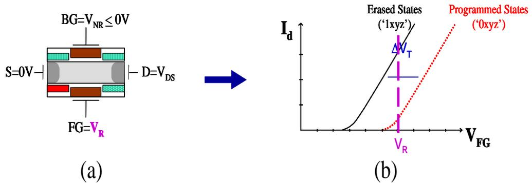
Figure 6.7: Identification of charge storage at Bit 1 of a 4-bit DG\_FET structure by the conventional method. (a) Bias conditions. (b) Resulting  $I_{DS}$ - $V_{FG}$  (constant  $V_{DS}$ ) curves, describing the separation between the programmed ('0xyz') and erased ('1xyz') Bit1 states.
