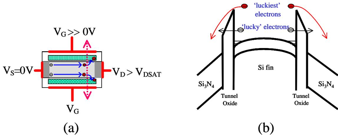
Figure 3.3: The HEI mechanism can be used to selectively program the bit next to the Drain electrode (Bit 2). (a) Bias conditions (b) Energy band diagram (through the dashed line in (a)), illustrating the HEI mechanism.
