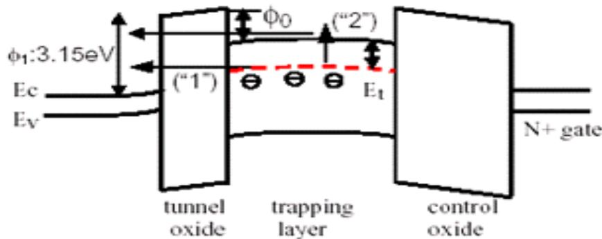
Figure 2.2: Energy band diagram through the gate-stack of a SONOS NVM cell while in retention mode ( $\phi_o \sim 1.03\text{eV}$ ).
