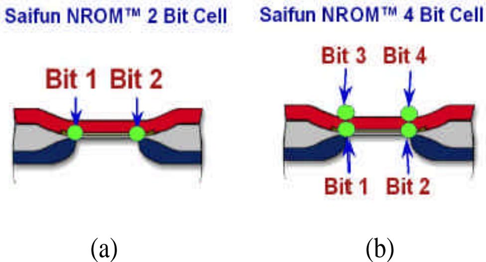
Figure 6.2: 2D Schematic view of Saifun’s (a) 2-bit, and (b) 4-bit NROM<sup>™</sup> NVM cells [6.4].
