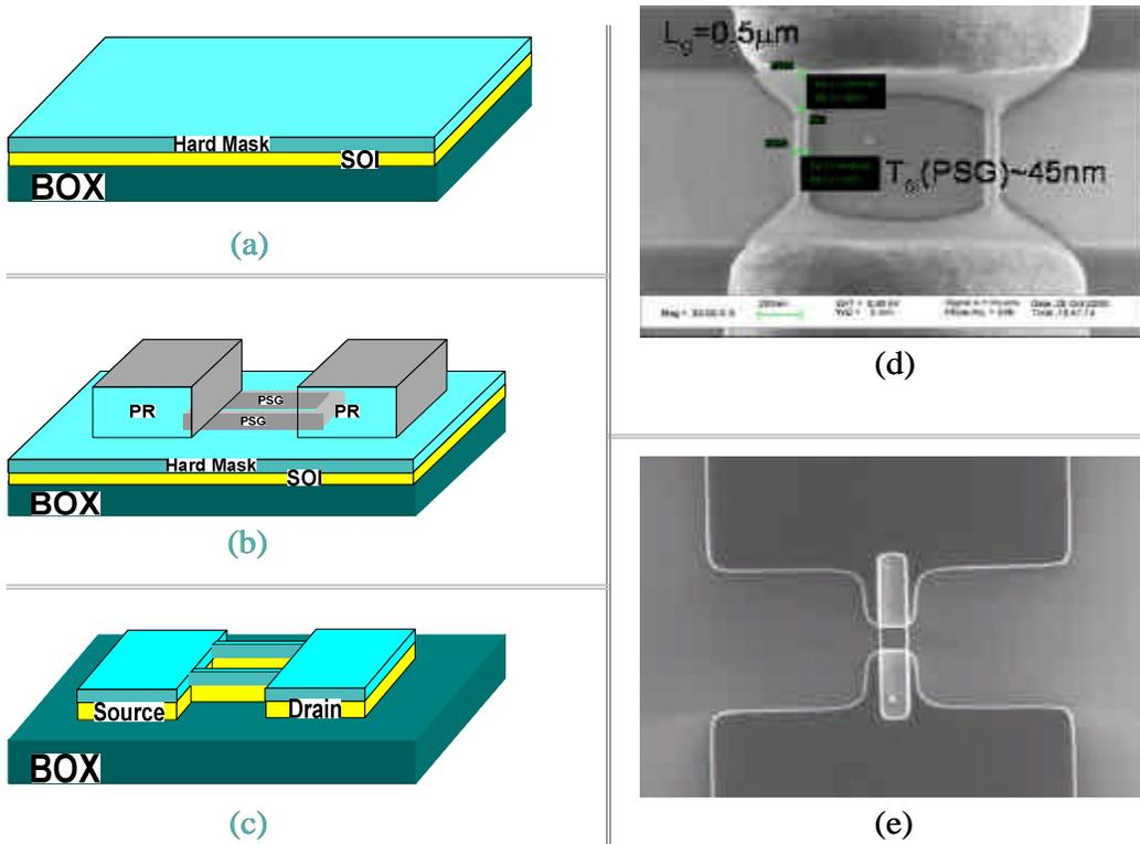
Figure 4.4: (a-c) Process flow used to fabricate gate-sidewall storage (GSS) FinFET NVM cells –ACTIVE Area Definition. (d-e) SEMs of a fabricated cell after completion of processing steps (b) and (c), respectively.
