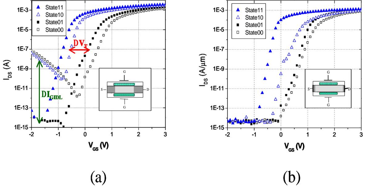
Figure 3.6: Simulated  $I_{DS}$ - $V_{GS}$  curves for (a) a gate-aligned (with  $L_g \sim L_{eff}$ ), and (b) a gate-underlapped (with  $L_g < L_{eff}$ ) SONOS FinFET NVM cell, showing that GIDL can be only be used in the former case to distinguish the state of Bit 2 ( $L_g=100\text{nm}$ ,  $T_{si}=40\text{nm}$ ,  $L_q=25\text{nm}$ ,  $V_{DS}=1.5\text{V}$ ).
