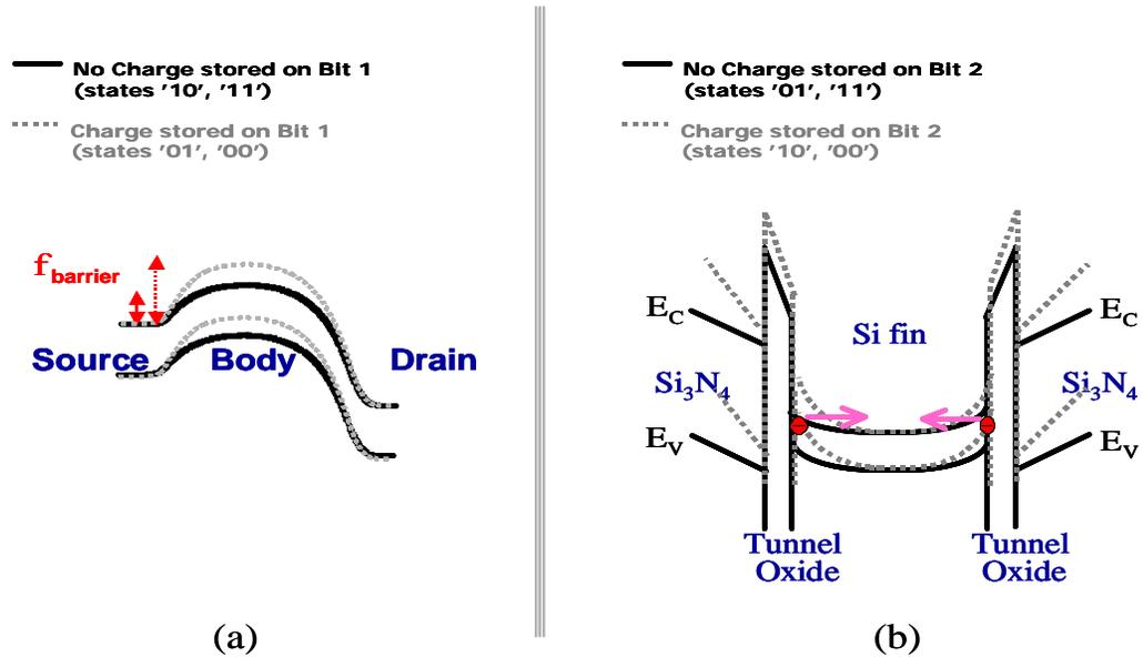
Figure 3.5: Energy band diagrams illustrating the charge detection methods that can be used with the FinFET SONOS NVM Cell: (a) charge stored on the bit next to the source electrode (i.e., Bit 1) affects the source-to-drain potential profile and thus the cell’s  $V_T$ . (b) Charge stored on the bit next to the drain electrode (i.e., bit 2) affects the cell’s transverse field (next to the Drain) and thus the cell’s GIDL current.
