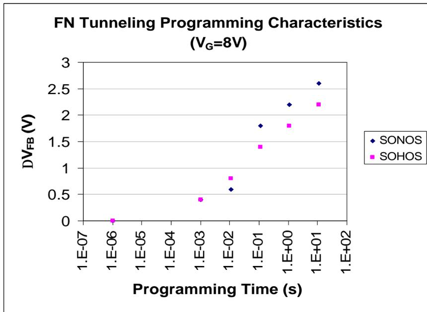
Figure 2.6: Programming Characteristics: Flat-band voltage shift ( $\Delta V_{FB}$ ) vs. programming time (at a gate voltage,  $V_G$ , of 8V) for both SONOS, SOHOS devices.
