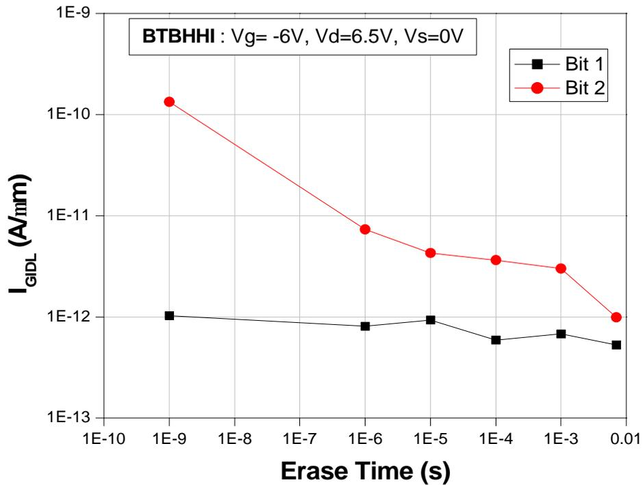
Figure 3.14: Bit2 BTBHII erase characteristics of the SONOS FinFET NVM cell (measured @  $V_{GS} = -1.5V$ , and  $V_{DS} = 1.5V$ ).
