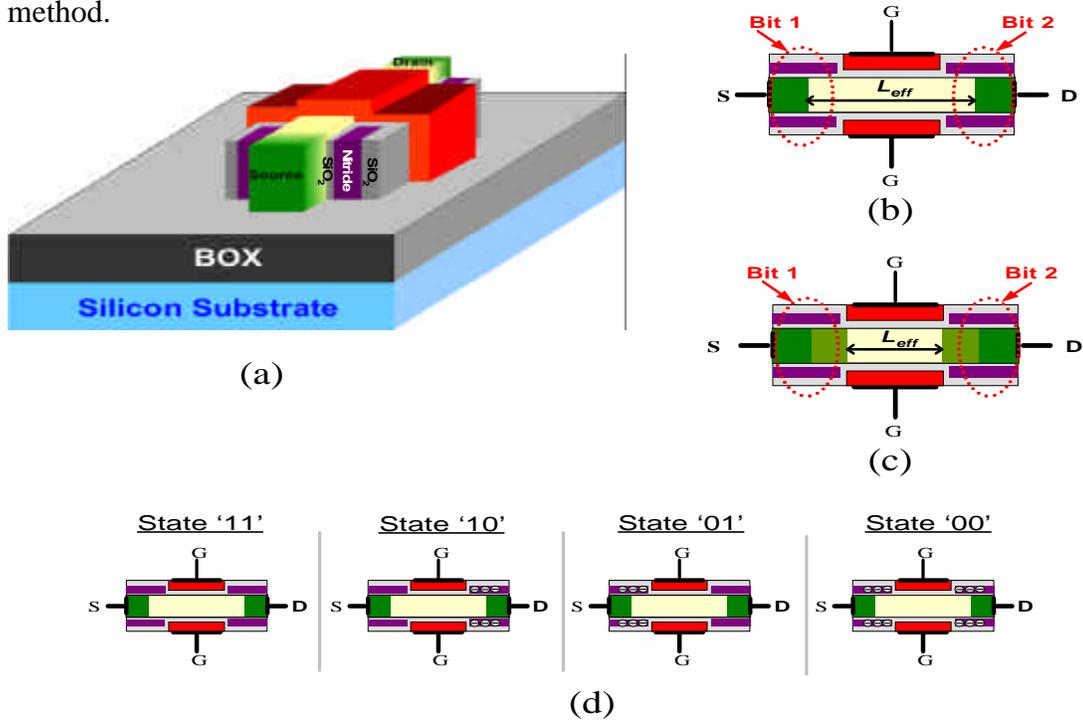
Figure 4.1: (a) Isometric view of the FinFET NVM cell with charge storage sites located at the gate sidewalls. The 2D schematic cross-sections of gate-underlapped ( $L_{eff} > L_g$ ) and gate-overlapped ( $L_{eff} \sim L_g$ ) cell structures are shown in (b) and (c), respectively. (d) Definition of the 4 charge-storage states of the dual-bit cell.
