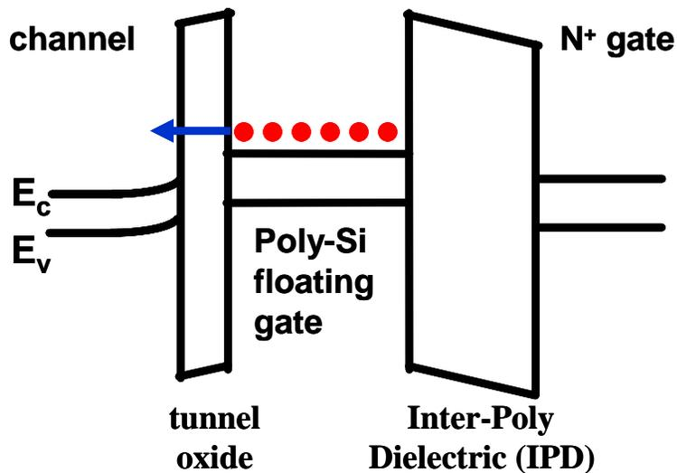
Figure 1.6: Energy band diagram of a floating-gate NVM cell during charge retention (i.e., with no voltages applied to a programmed cell). As shown, the stored electrons can (quantum-mechanically) tunnel back onto the channel (even with no bias applied to the structure).
