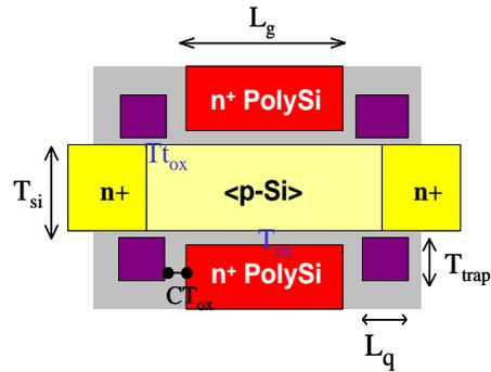
Figure 4.2: Parameter settings for Taurus 2-dimensional device simulations.
