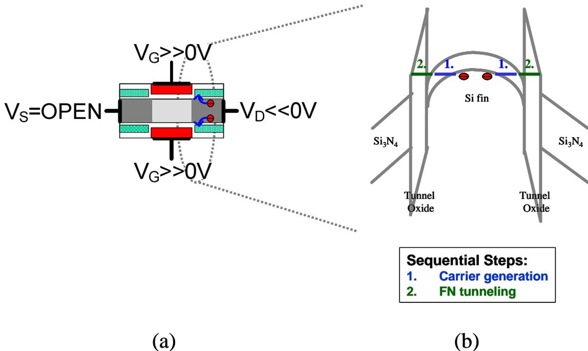
Figure 5.5: The band-to-band Hot Electron Injection (BBHE) programming mechanism [5.12],[5.14]: (a) Bias conditions. (b) Energy band diagrams (used to describe the mechanism).
