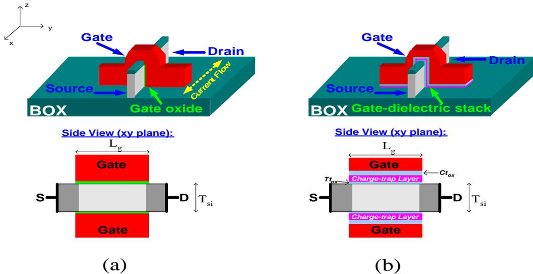
Figure 3.1: Isometric view (and 2D planar cross-section) of (a) the dual-gate FinFET transistor structure [3.4], and (b) the modified charge-trapping NVM FinFET structure, which essentially replaces its gate dielectric by a multi-layer stack.
