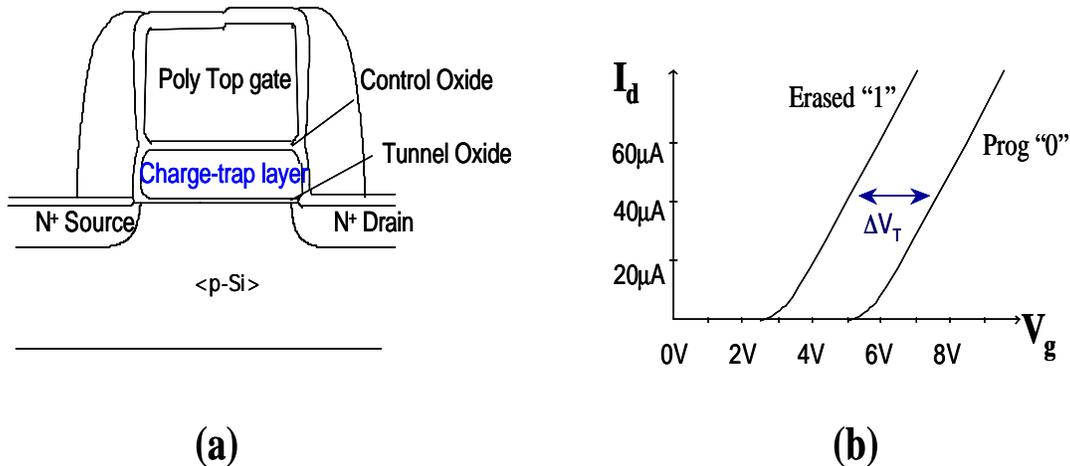
Figure 1.2: (a) Schematic cross-section of the conventional flash memory cell. (b) The storage of electrons within the charge-trapping layer modulates the cell's threshold voltage ( $V_T$ ), and this modulation can thus be used to detect charge storage (and hence the information stored within the cell).
