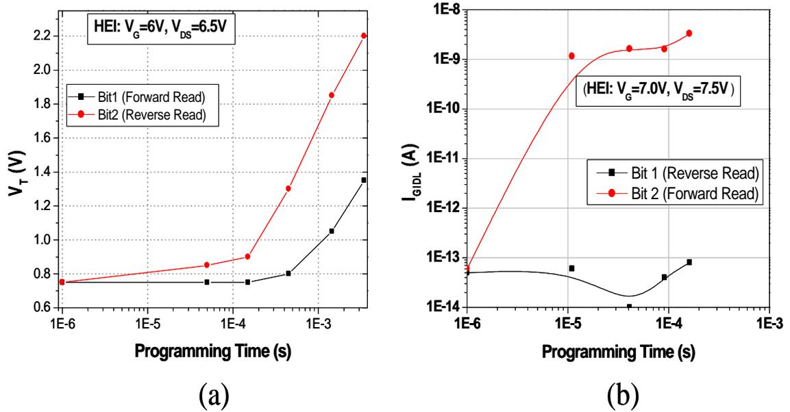
Figure 3.13: Bit2 HEI programming characteristics of a SONOS FinFET NVM cell, as measured by (a) the conventional ( $\Delta V_T$ ) and (b) the new ( $\Delta I_{GIDL}$ ) charge detection methods. In the latter case, the GIDL current of the programmed and erased states is measured @  $V_{GS} = -1.5V$ , and  $V_{DS} = 1.5V$ . The CBD effect in (a) is evident.
