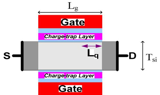
Figure 3.4: Parameter settings used in the 2-Dimensional (2D) Taurus device simulations on an optimized SONOS DG-FET structure with  $L_g=100$ nm.
