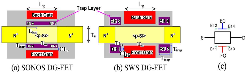
Figure 6.4: Schematic cross-sections of (a) the conventional SONOS, and (b) the Sidewall Storage (SWS) 4-bit DG-FET NVM cell designs. (c) Symbolic representation for either structure.
