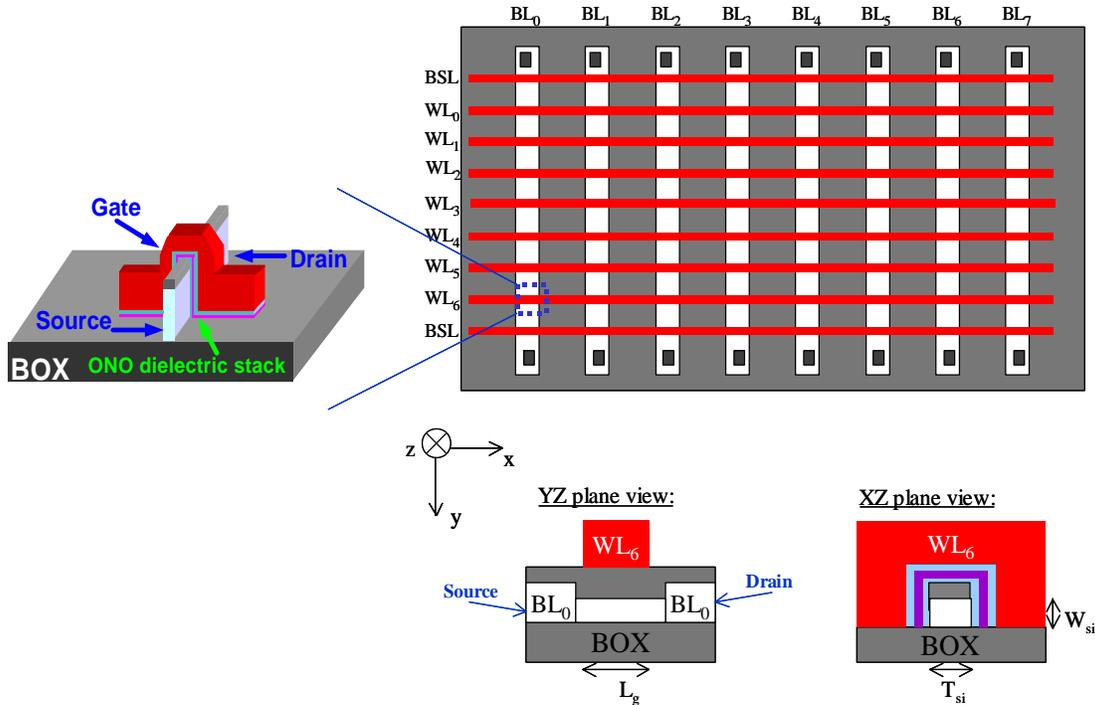
Figure 3.18: Basic schematic layout (not to scale) and cross-sections of the NAND-type array architecture that utilizes the dual-bit SONOS FinFET NVM cell as its unit cell (highlighted within the layout with a dashed line).
