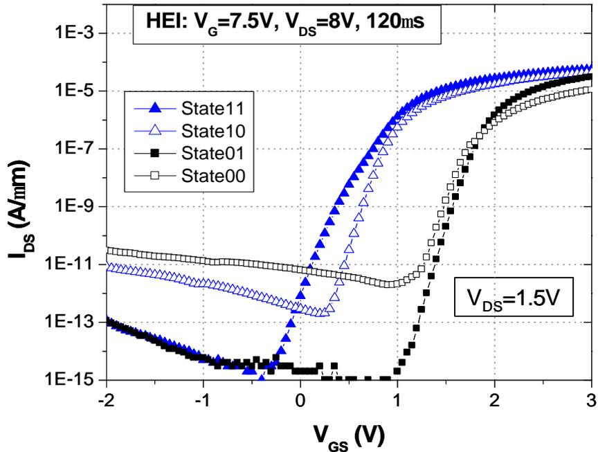
Figure 3.12: Measured SONOS FinFET cell  $I_{DS}$ - $V_{GS}$  characteristics ( $V_{DS}=1.5V$ ) for each of the 4 programmed states ( $L_g=350nm$ ,  $T_{si}=50nm$ ).
