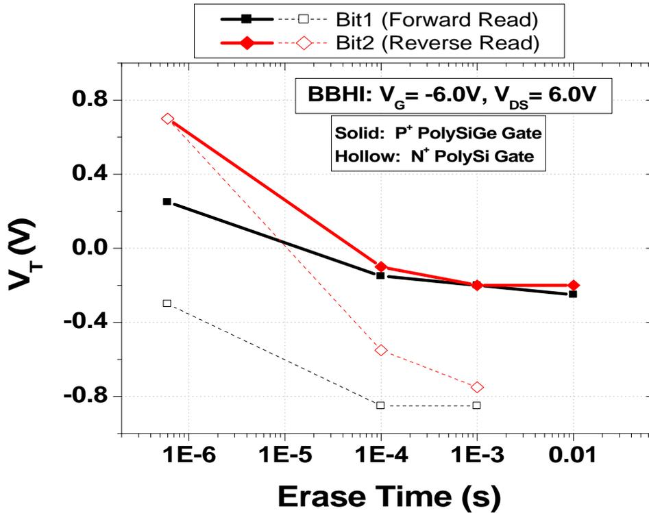
Figure 5.9: Band-to-band Tunneling-induced Hole Injection (BBHI) Erase characteristics of a p-channel GSS FinFET NVM cell.
