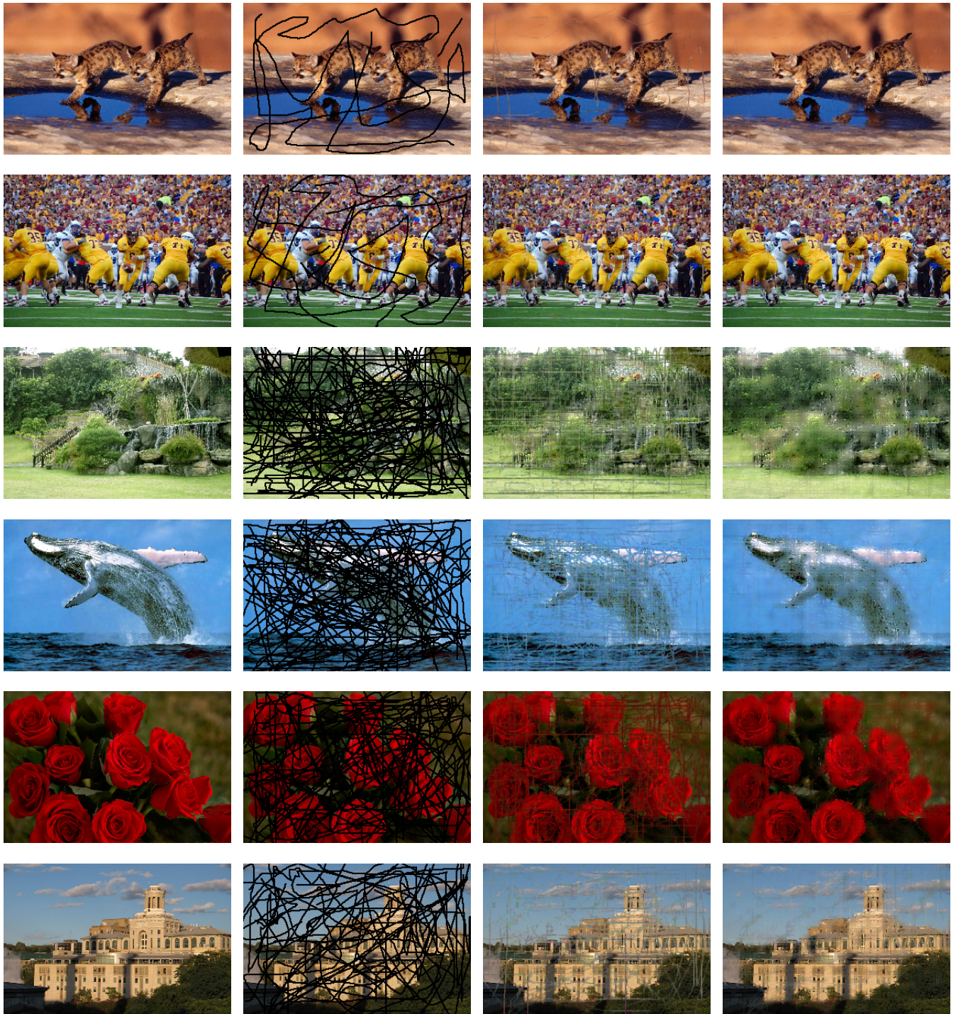
Figure 8: Image restoration results using PMF and KPMF (best viewed in color). From left to right: original images, corrupted images (regions to be restored are in black), images restored using PMF, and images restored using KPMF. For KPMF, \Delta equals to 5 when constructing the row and column graphs, and Diffusion kernel with \beta = 0.5 is used to obtain the kernel matrices.
