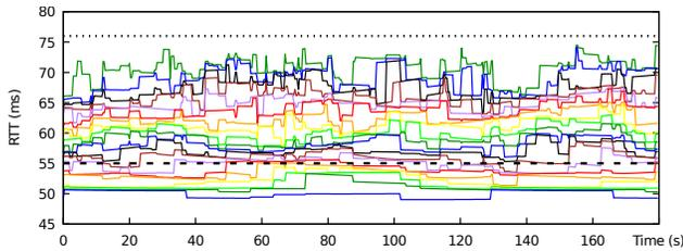
Figure 11: Phase 2 Multipath RTT, NYC-LON, best 20 disjoint paths.
