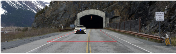
Figure 3: Annotation trapezoid. User adjusts the four corners that represent the valid sampling subspace of x and z . The size of the car scales according to how close it is to the vanishing point.
