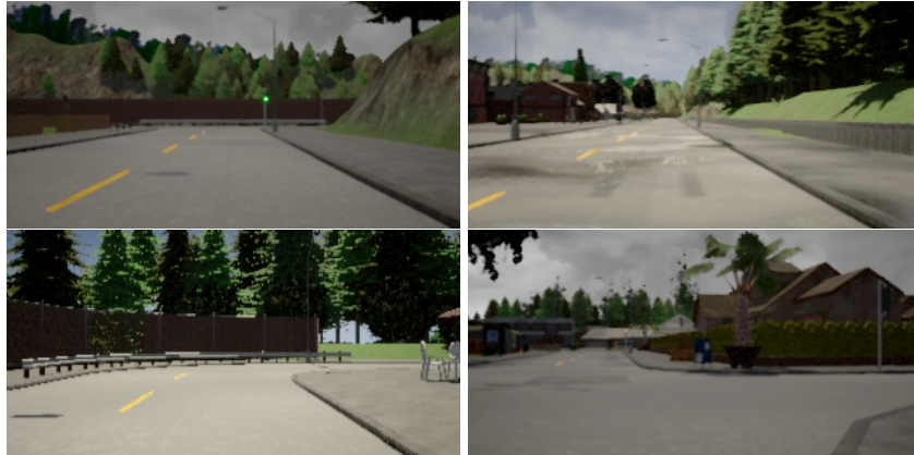
Fig. 1. Example input images to the neural network, rendered in CARLA, showing a variety of orientation, weather, and road conditions.
