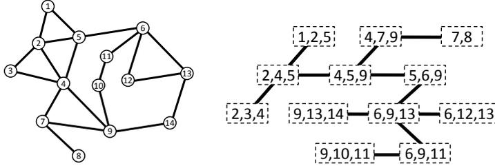
Figure 1: The IEEE 14-bus power network (left figure) and its minimal tree decomposition (right figure).
