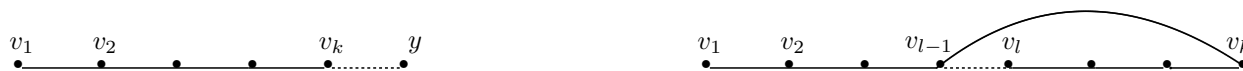
Figure 14.2: On the left is shown operation extend(P, y) , which adds vertex y to the end of the path. On the right is shown operation rotate(P, y) , which adds the edge from v_k to y = v_{l-1} and removes edge (v_{l-1}, v_l) .
