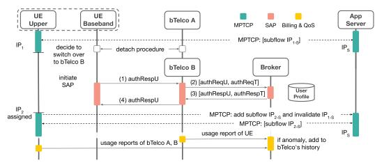
Figure 4: An overview of the attachment, mobility, and billing/QoS process in CellBricks depicting the key events and message exchanges happen during the SAP, MPTCP, and billing protocol over time. Note that authReqU/T and authRespU/T are defined in Fig.2 and Fig.3.
