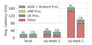
Figure 7: Latency breakdown by module in the Magma baseline (BL) and CellBricks (CB) during an attachment request.
