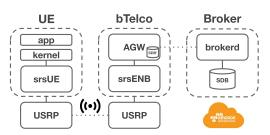
Figure 6: An overview of our testbed. AGW: access gateway; SDB: SubscriberDB.
