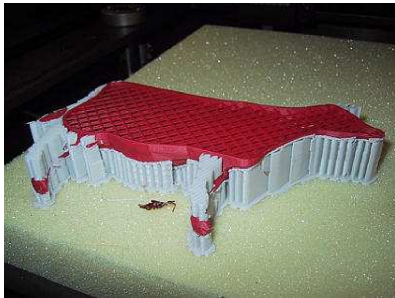
(c) Thin-walled cow model being built on an FDM machine
