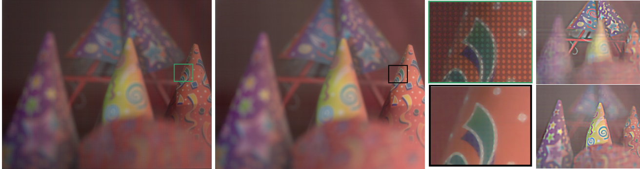
Figure 1: Our heterodyne light field camera provides 4D light field and full-resolution focused image simultaneously. (First Column) Raw sensor image. (Second Column) Scene parts which are in-focus can be recovered at full resolution. (Third Column) Inset shows fine-scale light field encoding (top) and the corresponding part of the recovered full resolution image (bottom). (Last Column) Far focused and near focused images obtained from the light field.
