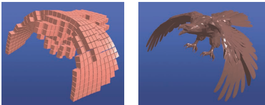
Figure 8: Eagle surface mesh (right) for which a cube mesh was generated (left) to simulate elastic deformation.
