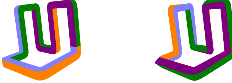
Figure 3: (a) The forward projection used for the rotation minimizing frame causes the starting and ending frames to misalign. (b) Gradually adding in 180^\circ of twist across the sweep causes the frames to align.
