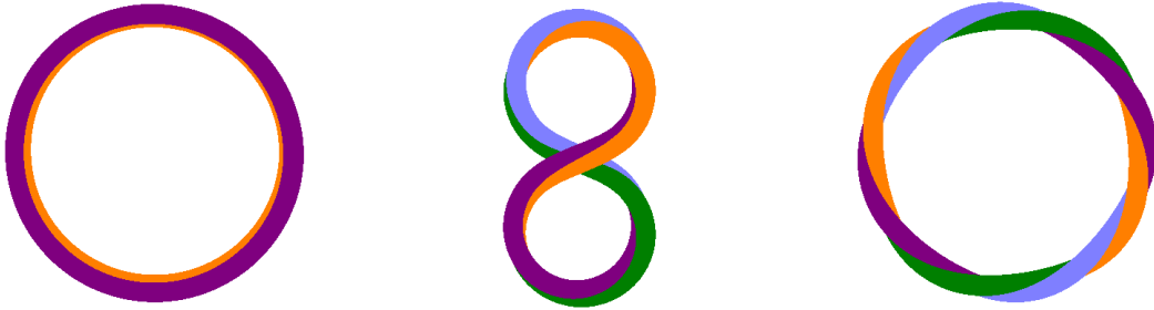
Figure 2: The full figure-8 cross-over move adds \pm 720^\circ of torsion: (a) Circular start configuration with zero torsion; (b) Figure-8 with 360^\circ of twist; (c) Circular end configuration with 720^\circ of twist.
