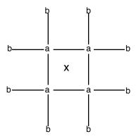
If you imagine the degenerate case where one dimension is much larger than the other, we feel that the scheme should morally reduce to one-dimensional cubic interpolation, with weights -1/16 on the "outward" points and 9/16 on the "inward" ones. If we divvy those weights equally amongst the *a*s and *b*s, we find that each *a* should have weight 5/16 and each *b* weight -1/32.
