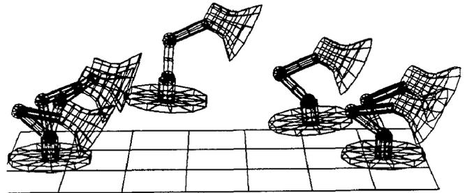
Figure 4: A variation on the basic jump in which the contact force on landing is constrained to be small. The force of impact is reduced by squashing just before landing, reducing the velocity and hence the kinetic energy of the base. In contrast, the jump in Figure 3 exhibits a slight *stretch* before impact, producing an energy-absorbing stomp.
