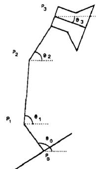
Figure 2: Luxo's parameters:  $\mathbf{P}_0$  is a translation, and  $\theta_i$  is the orientation of the  $i$ -th link. Points  $\mathbf{P}_1$ - $\mathbf{P}_3$  are computed from these parameters.
