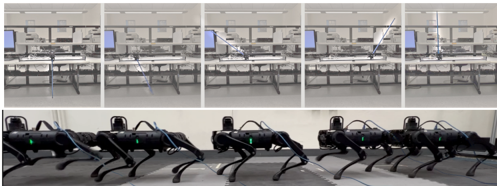
Figure 1: We learn precise stabilizing policies on hardware for the Quanser cartpole [1] (top) and the Unitree A1 quadruped [2] (bottom) using only seconds and a few minutes of real-world data, respectively. A video of our experiments can be found here https://youtu.be/17kBfitE5n8
