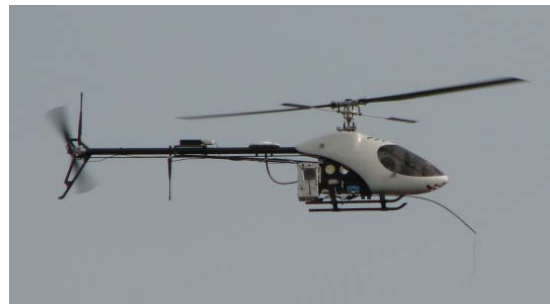
Figure 4. A UAV testbed with flight control software enabled with model-predictive algorithm (UC Berkeley, 2006)
