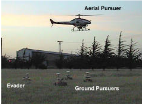
Figure 10: The Berkeley AeRobot testbed for multi-agent: One UAV and two UAVs vs. One UGV deployed for a pursuit-evasion game
