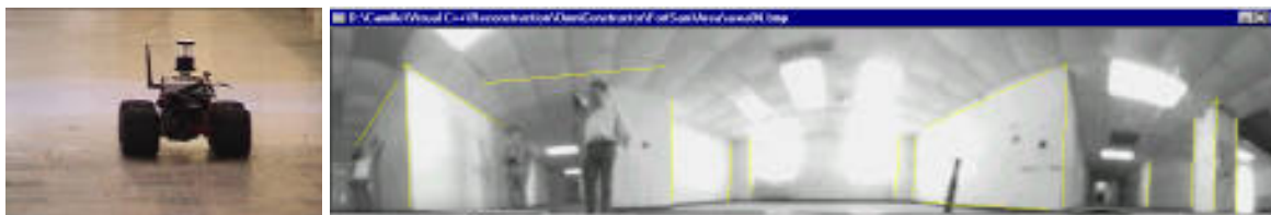
Figure 5: A panoramic view (right) obtained from the omnidirectional camera mounted on the robot (left).
