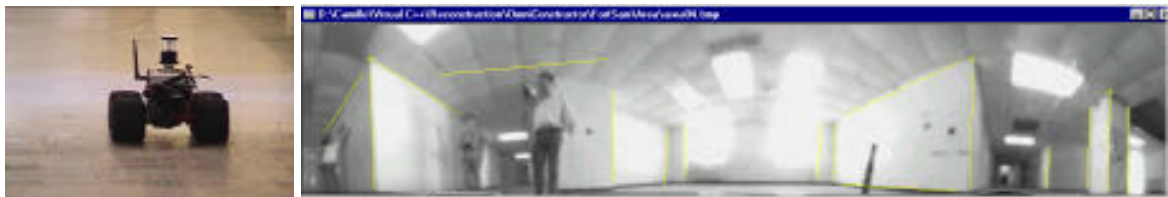
Figure 5: A panoramic view (right) obtained from the omnidirectional camera mounted on the robot (left).
