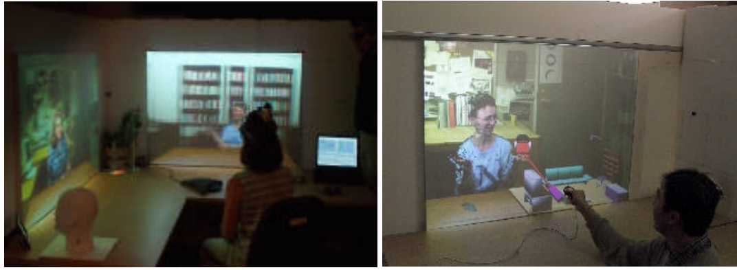
Figure 7: A user in Chapel Hill (left) wearing polarized glasses and an optical tracker communicates with two remote users from Philadelphia and Armonk. The stereoscopically displayed remote 3D-scenes are composed from incoming streams of textured 3D data. A user in Chapel Hill (right) wearing the same devices interacts in a mini office model which is virtually shared with the remote user in Armonk (Courtesy of UNC-UPenn)
