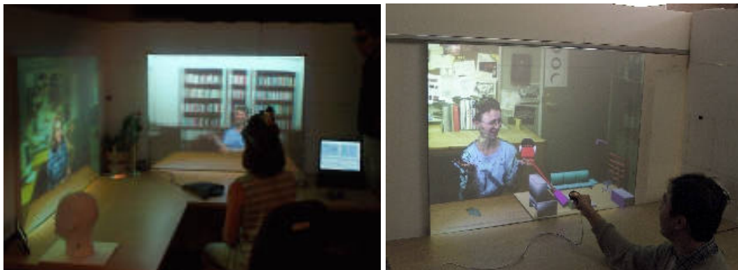
Figure 8: A user in Chapel Hill (left) wearing polarized glasses and an optical tracker communicates with two remote users from Philadelphia and Armonk. The stereoscopically displayed remote 3D-scenes are composed from incoming streams of textured 3D data. A user in Chapel Hill (right) wearing the same devices interacts in a mini office model which is virtually shared with the remote user in Armonk (Courtesy of UNC-UPenn).
