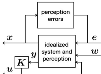
Figure: The robust control view of the closed-loop system
