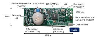
Figure 1: Hamilton, a single board that has a low-power 32bit SoC and provides 7 types of sensors.
