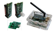
(a) WSN ecosystem: 1) with 6 sensors, 2) with 7 sensors (+PIR sensor), 3) small powered router, and 4) border router with a raspberry pi
