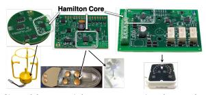
(b) Extended ecosystem: 1) ultrasonic anemometer, 2) auto-heating/cooling insole and smart desk fan (both with an actuator), and 3) thermostat
