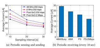
Figure 8: Average current consumption of Hamilton/RIOT/OpenThread with various settings.
