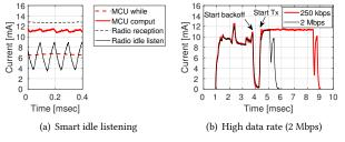
Figure 3: Current waveform of various Hamilton operations, demonstrating the impact of Hamilton's advanced radio features on power consumption.
