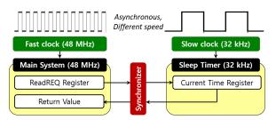
Figure 5: An example of interaction between different asynchronous clock domains (the case of SAMR21).
