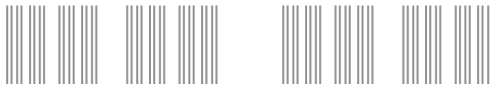
Fig. 8. The priority message bits are used to refine a point on a Cantor set. The natural tree structure of the Cantor set construction allows us to encode bits sequentially. The Cantor set also has finite gaps between all points corresponding to bit sequences that first differ in a particular bit position. These gaps allow us to reliably extract bit values from noisy observations of the Cantor set point regardless of which point it is.
