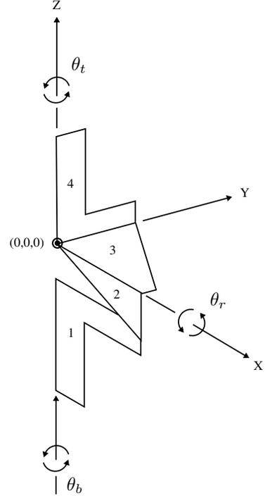
Fig. 10. Kinematic representation of the wing differential mechanism.
