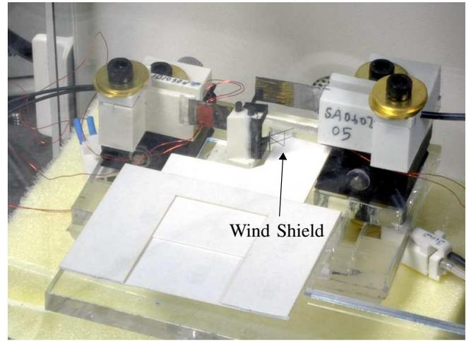
Fig. 4. Closeup of lift measurement setup for  $06-\beta$ .
