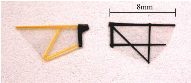
Fig. 3. Previous polyimide spar wing (left) and new carbon fiber spar wing (right).
