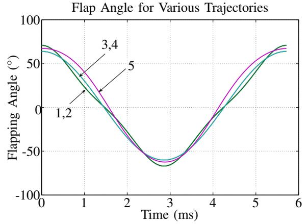
Fig. 11. Comparison of flapping angle obtained in the five trajectories.
