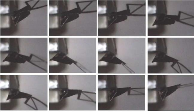
Fig. 6. Top view wing trajectory of 06- $\beta$ .
