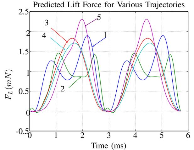
Fig. 13. Comparison of predicted lift forces obtained from various trajectories.
