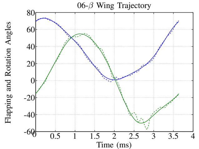
Fig. 5. Wing trajectory for  $06-\beta$ . Flapping angle is the top trace, rotation angle is the bottom. Raw data is plotted with a dotted line, filtered data with a solid line.
