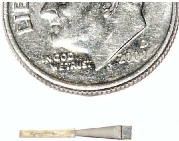
Fig. 10. Piezoelectric bimorph actuator for MFI.
