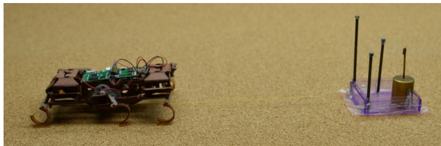
Figure 2.8: Sled with a weight in it being pulled by a VelociRoACH with spines on corkboard.
