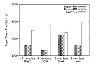
Fig. 11: Average Reply Time - Transfer: HAVEN outperforms HAProxy by a factor of 2.1
