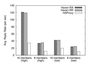
Fig. 12: Average Reply Rate (per second): HAVEN outperforms HAProxy by a factor of 3.8
